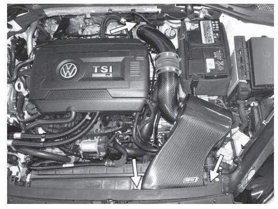
31) Reinstall the air intake assembly onto the car. Attach the vacuum line to the port on the bottom of the intake. Install the right front tab of the intake into the mounting slot on the back of the radiator core support. Push the rubber grommet on the bottom of the intake down on the mounting post. Install the screw on the left side of the intake to the back of the core support. Finally, connect the back pipe to the turbo inlet pipe and secure with the hose clamp.
