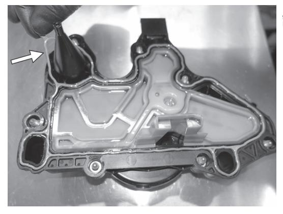
13) Carefully lift and remove the gasket from the bottom of the factory PCV top plate.
