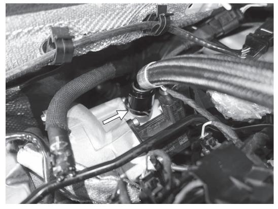
27) Take the APR catch can hose with the quick disconnect fitting, and push it down on the port on top of the turbo inlet pipe. Slide the clip in to lock the fitting on the turbo inlet pipe port.
