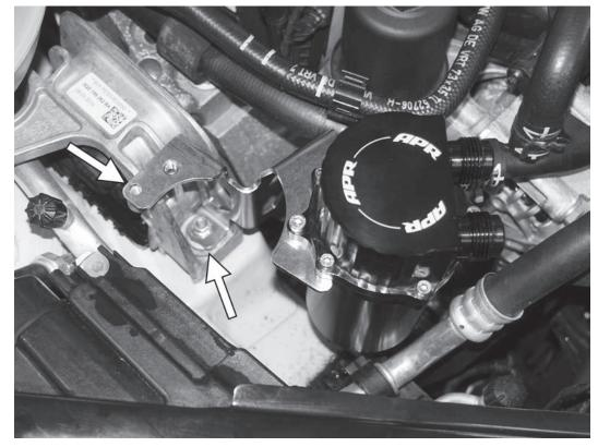
23) Install the APR catch can assembly in the car, attaching it to the factory engine mount. The lower hole in the bracket goes onto the threaded post on the engine mount, and is secured with the supplied 10mm flanged nut. One of the upper holes on the APR bracket will align with the mounting hole location for the factory windshield washer reservoir.
