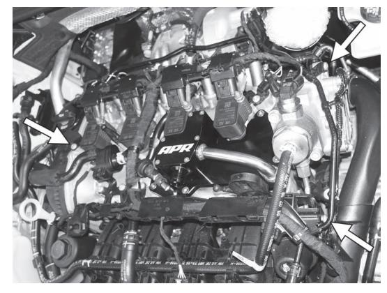
21) Reinstall the factory coolant line that runs along the back and side of the engine with the three original T30 screws. Secure the screws to 9Nm (80 in-lbs).
