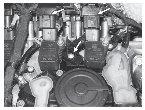
5) Disconnect the electrical connectors to all four ignition coil packs. Remove the T30 screw from the back of the factory PCV plate.
