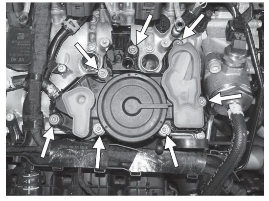
9) Remove the seven T30 screws holding the PCV top plate to the top of the cylinder head.
