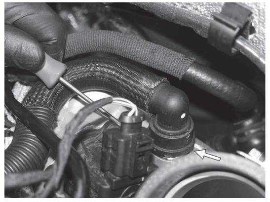
7) Using an angles pick tool, work the pic around the bottom side of the PCV connection on the turbo inlet pipe. Remove the connection from the pipe, and remove the hose from the car.
