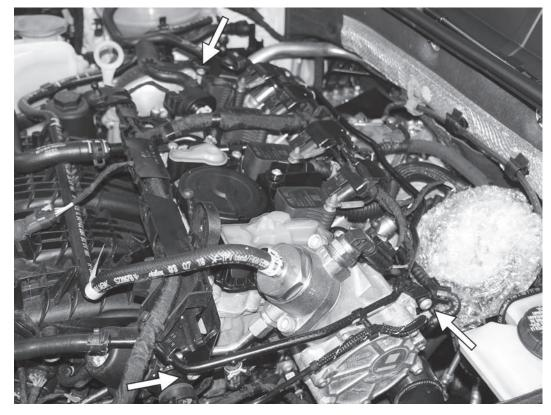
3) Remove the three T30 screws that hold the hard coolant pipe that runs along the back and left side of the cylinder head.
