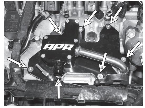
15) Install the APR top plate onto the top of the cylinder head cover. Install the seven 4MM allen screws. A ball end allen wrench will be needed for the one screw underneath the catch can hose fitting. Once all the screws are installed, torque them in the pattern shown to 9Nm (80in-lbs).
