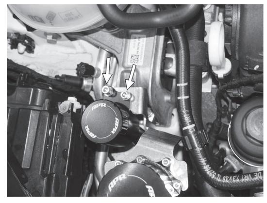
25) Mount the APR washer filling cap to the previously installed APR bracket with the two supplied 5mm allen screws. The washer fluid can be topped off if desiired.
