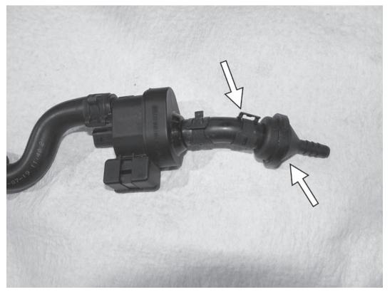
17) Insert the supplied check valve and spring clamp onto the rubber hose on the end of the N80 valve. Be sure to put the tapered side of the check valve away the N80 valve.
