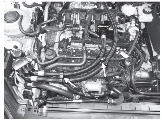
29) Attach the two supplied hose management clips to the catch can hoses. Ensure the lines are routed correctly, are not under tension, and do not rub on other hoses or lines before tightening the clamps in place with a 4.5MM hex wrench.
