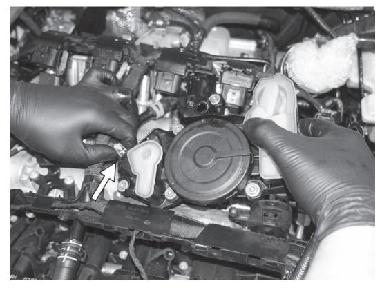
11) Lift and remove the PCV top plate from the cylinder head cover, disconnecting the rubber hose from the right side as shown.
