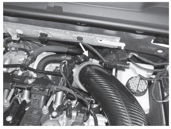
1) Raise the hood and remove the engine cover by pulling up on each of the four corners of the cover. Loosen the hose clamp connecting the rear air intake tube to the turbo inlet pipe.
