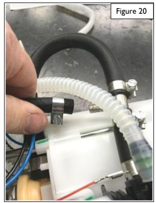
19. Tighten all the hose clamps and be sure all the wire plugs are connected and seated. The final assembly will look like Figures 21 and 22.
