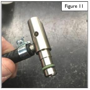
II. Install the Dinan tee to the end of the regulator in the lid as shown. There is a slot in the tee that aligns with a tab on the regulator. As you install it, also feed the other end of the hose through the 1/2" hole you drilled. See Figures 12 and 13.
