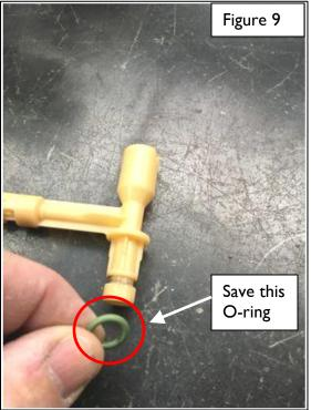
10. Transfer the O-ring to the groove on the Dinan Internal Hose Assembly #1, as shown on Figures 10 and 11.
