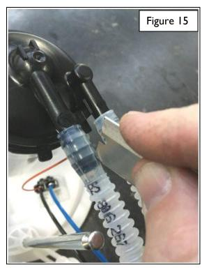
15. After removing the stock fuel line, reinstall the fuel filter half of the assembly onto the lower cup section using the spring and attaching it with the small E-clip (see Figure 16).
