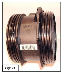
28. Install the Air Mass Meter into the Dinan lid using the supplied Phillips head selftapping screws and rectangular washers. See figures 22 and 23.
