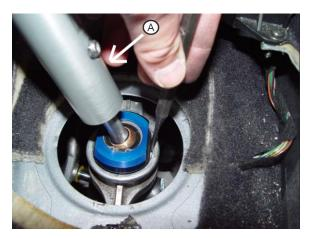
12. Replace selector arm through bottom of shifter. Place included washers on either side of Dinan shifter. Replace U-clip.
