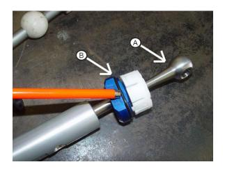
II. Place the shifter assembly into the carrier of the car with the bend towards the driver's side/rear of the car. Gently tap the tabs of the ball-clamp until they snap into the carrier. Ensure that ball-clamp is securely affixed to the carrier.
