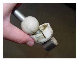
9. Place ball-clamp onto Dinan shifter pivot cup. Align so that tabs of the ball-clamp are underneath the bolt head and nut on the shift lever.
