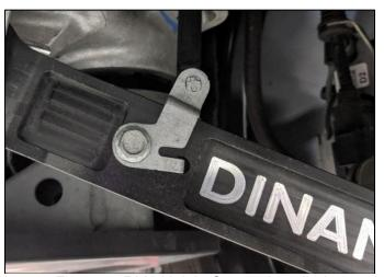
Figure 4: Ride Height Sensor Installed
