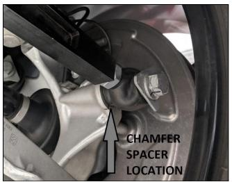
Figure 2: Chamfer location for Toe Link
