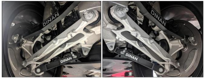
Figure 1: Rear Left Suspension Links (LEFT) and Rear Right Suspensions Links (Right)
