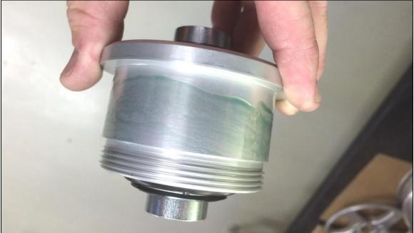
4. See figure below. Slide the ball joint assembly into the control arm. Threads shall be inserted first from the side that has the alignment arrow on the control arm. While inserting use a slight turning motion to further spread the Loctite around. Align the arrow on the ball joint assembly with the arrow on the control arm. The ball joint assembly should sit flush to the control arm.
