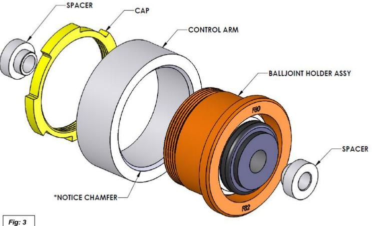
5. Install the Dinan retaining cap onto the arm. Put a small amount of Loctite on the internal threads of the cap and torque to 110 foot-pounds to secure the retaining cap. A special Dinan cap tool is included in every kit. This tool is used with a 1/2" torque drive. Set torque wrench to 110 foot-pounds and do not concern yourself with a conversion factor. See Figure 4.
