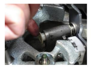
Reconnect the small metal circular clip to the center shaft of the side-to-side linkage to secure it in place and tighten the 13mm nut onto the threads of the splined selector shaft for the front-to-back linkage.
