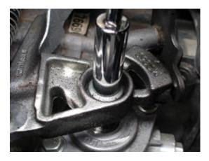
Once the 13mm nut is removed, slide the front-to-back linkage up off of the splined selector shaft. This will take some force and it is recommended to rock the linkage from side to side very slightly in order to loosen it, but please do not use a hammer or anything else to pound or tap the shaft out of the bottom of the linkage as this may lead to damage to various components. Though it will take some effort, the linkage will certainly come loose within a short time.
