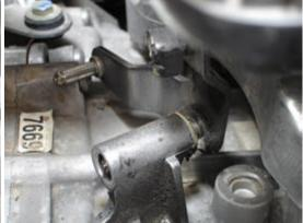
Once the white plastic guide has been freed from the front-to-back linkage and the side-to-side linkage has been tilted back against the transmission casing, it can be removed from the pivot mount. Please be certain that you also remove the second white plastic center pivot bushing as both of them will be reused later.
