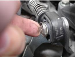
Also remove the small circular clip from the center pivot of the side-to-side linkage component.
