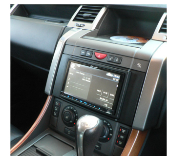
Fit the head unit into the cage, then fit the replacement panel.
