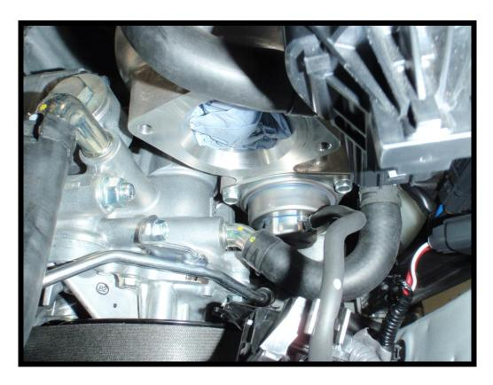
14. Install the new recirculating value through the gap between the radiator and body work. Bolt in position with bolts supplied in the kit and reconnect the vacuum hose.
