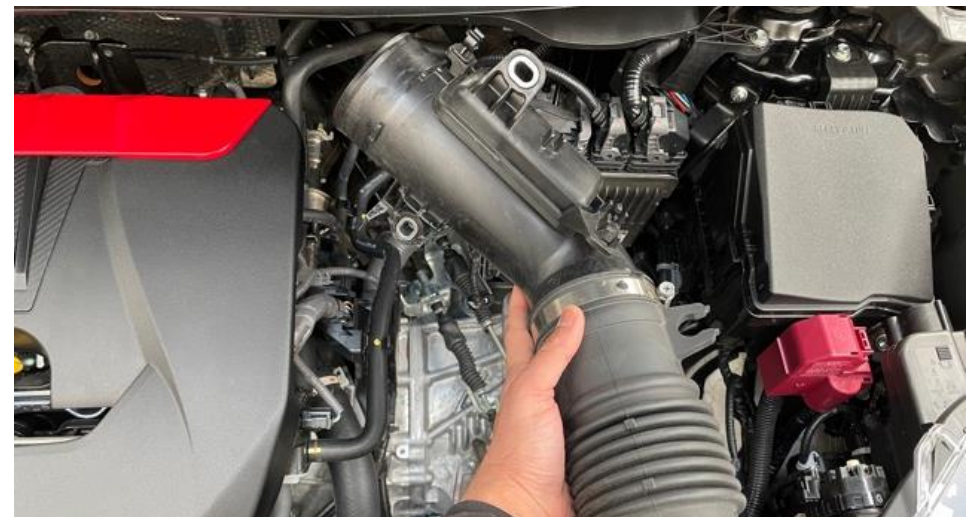
12. Remove the tube from the engine bay.
