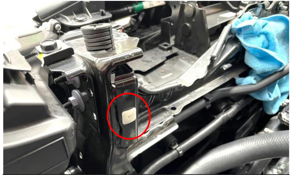
26. Insert the supplied white plastic clip into the square hole in the bodywork underneath the bonnet stop.
