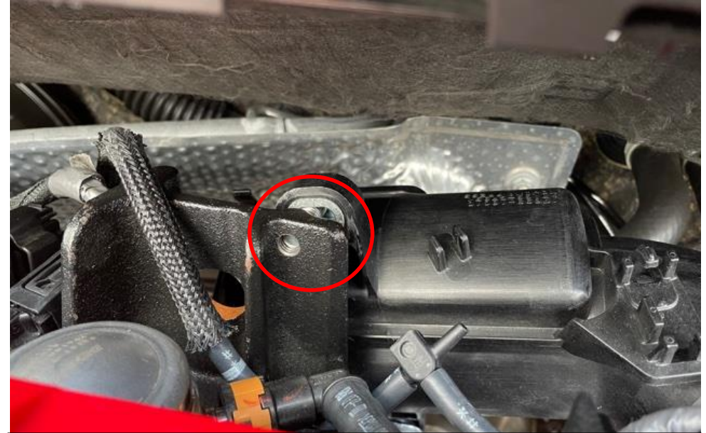
10. Move the vacuum line out of the way and remove the M8 bolt holding the top of the tube in place. There is also a second 13mm bolt on the lower side of the tube – remove this also (cannot be seen in the photo).
