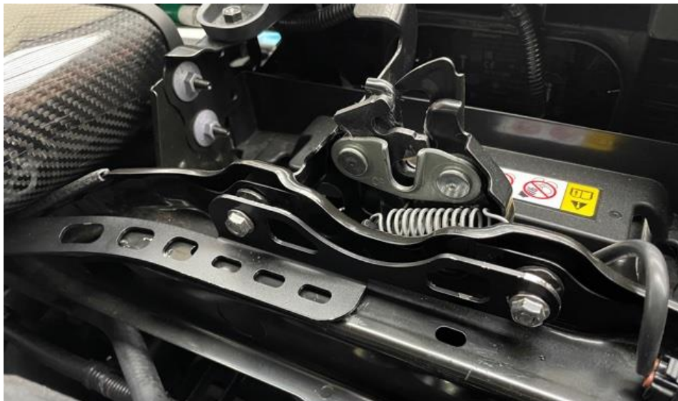
39. Secure the bracket by inserting 2 x M6 nuts onto the new bolts.
