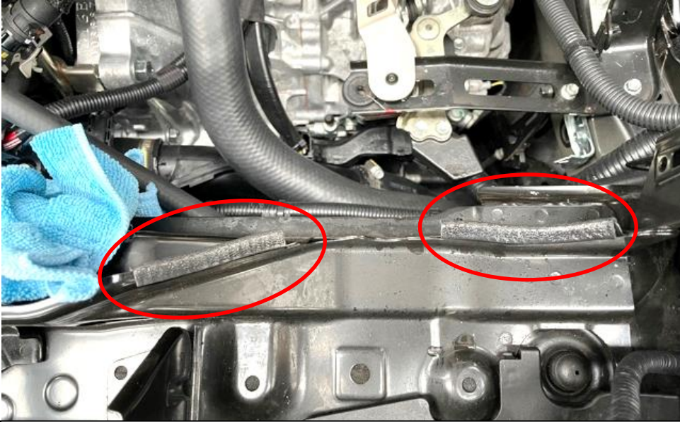
25. Push the 2 rubber strips onto the bodywork where the duct will be positioned.
