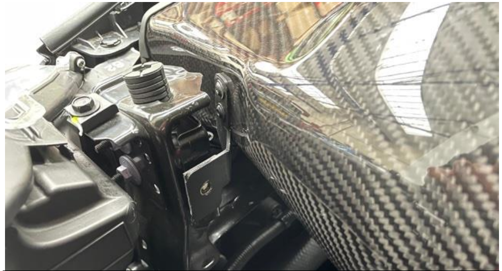
30. Position the bracket in front of the white clip.
