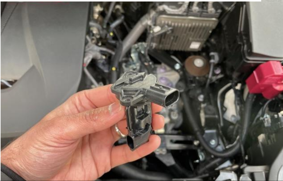
13. Remove the MAF Sensor from the airbox.
