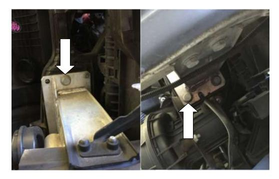
5. Install the x2 service bolts (M10 x P1.5mm x 120mm) in each side of the crashbar in the lower outside bolt hole. Then remove the remaining bolts.
