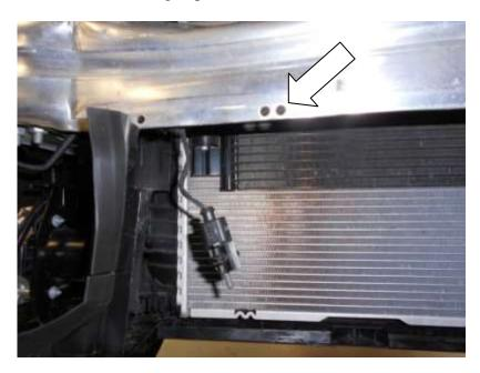
8. Moving to the right-hand side of the vehicle. Disconnect the headlight washer coupler and drain fluid into a suitable container.
