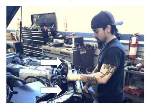
13. Use a 16mm socket and suitable ratchet to rotate the tensioner to release the tension on the belt and remove it.
