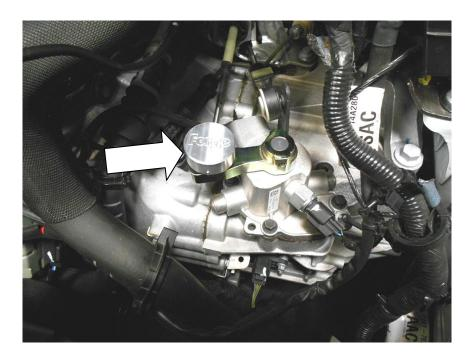
17. Using a suitable Allen key tighten the 3x grub screws.
