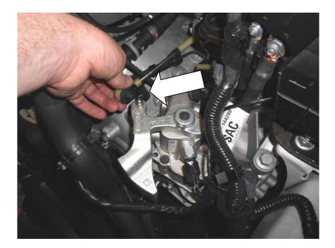
8. Place the Forge pin removal tool in position and using 5mm Allen key tighten to remove the locking pin.
