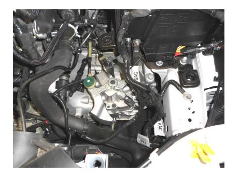
7. Using a 12mm spanner or similar tool, disconnect the control cable knuckle.
