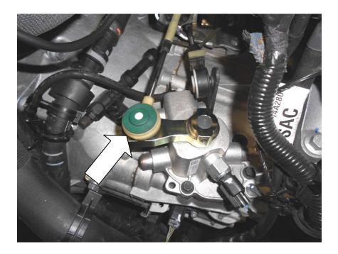
16. Place your Forge Slop reducer over the ball joint. Push down firmly to correctly seat the cap.
