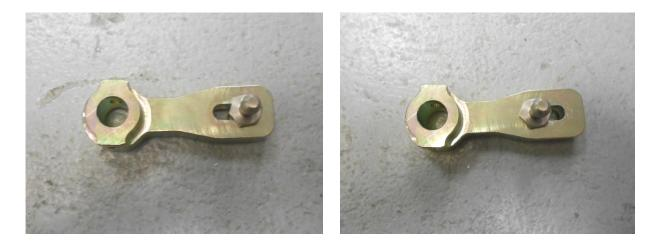
11. Start the split pin on a solid surface before fitting in to the gearbox shaft.
