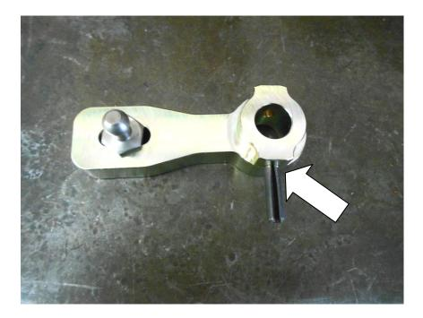
12. Mark the top of the gearbox selector shaft with a marker pen or similar showing the position on the locking pin hole.
