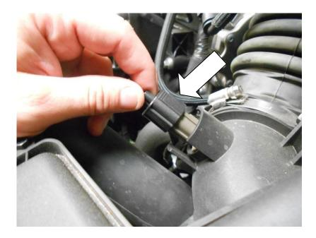
4. Unclip the upper and lower rubber intake scoop.
