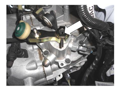
14. Using a small hammer drive the split pin into the Quickshifter until it is flush with the outside.
