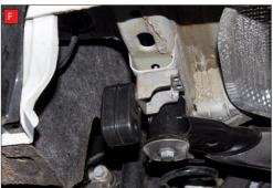
Scorpion Exhaust, fully tighten up all clamps and fixing and plug in the electronic valve motors.
