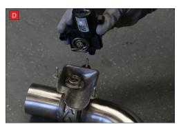
spring (This must stay on the electronic valve motor to work with Scorpion Exhaust).
