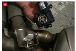
A) After you have removed O.E exhaust you will need to swap the valve motors to the Scorpion exhaust. Remove the 3 nuts ( keep safe as you will need them to bolt the electronic valve motor to Scorpion Exhaust).
