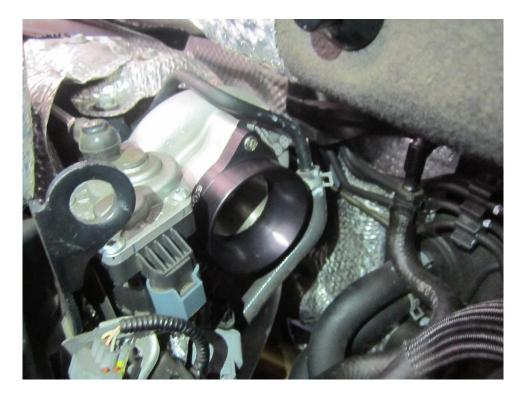
6. With the machined adaptor fitted to the turbo, you can now fit the Forge silicone inlet hose. Use the 70-90mm hose clamp provided to secure the inlet hose to the adaptor, fit it loosely at this stage to allow for adjustment.
