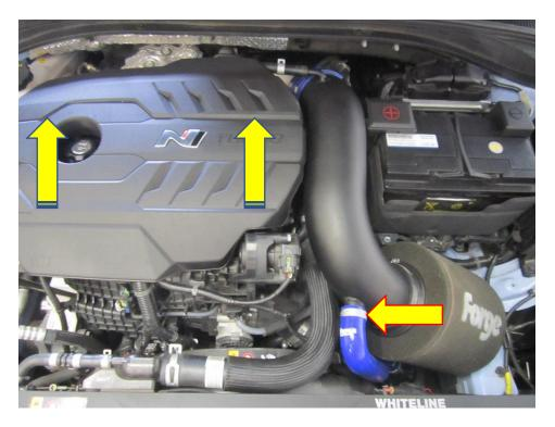
2. Remove the two breather hoses at the top of the intake pipe, like the previous step release the hose clamp to allow the hoses to be removed. Remove the 10mm fastener which secures the boost pipe to the engine. Finally undo the hose clamp attaching the silicone hose to the OE turbo elbow, use a 7mm socket and ratchet to do this. The intake pipe can now be removed from the vehicle.
