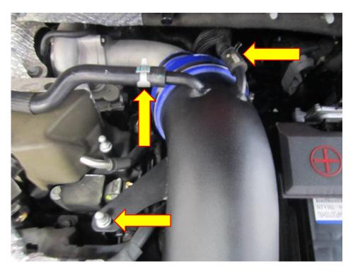
3. To remove the OE turbo elbow, using a 10mm socket and ratchet with extension remove the three 10mm fasteners attaching the elbow to the turbo, unclip the wiring harness attached to the turbo elbow, the turbo elbow can now be removed from the turbo. Be careful not to lose the OE gasket down the back of the engine bay when removing.
