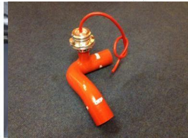
Fit new "T" piece and valve Fit valve and vacuum hose
