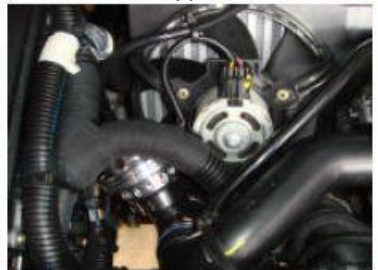
With the Valve installed tighten all clamps and secure the vacuum hose with the tie wraps supplied.
