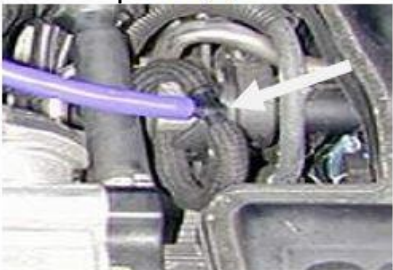
Remove the Hose from the hard pipe New Forge hose completely replaces stock hoses
