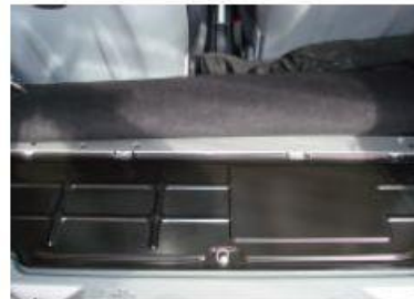
After checking that all tools have been removed replace the engine cover
