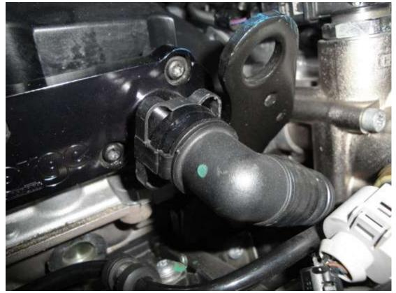
6. Using a 10mm socket and matching ratchet undo the 10mm bolt holding the plastic washer bottle pipe in place. Once the bolt is removed you will need to pull up on the bottom of the pipe to release it from the washer tank.
