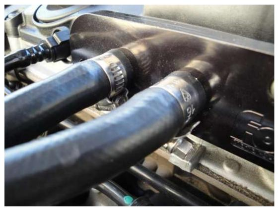
Install the Clip on blanking cap for the intake manifold. Prior to doing so, you will need to fit all 3 grub screws into the blanking plug unless you require a vacuum pipe if you are running a boost gauge. It is recommended that when fitting the grub screws, use a semi permanent thread lock.
