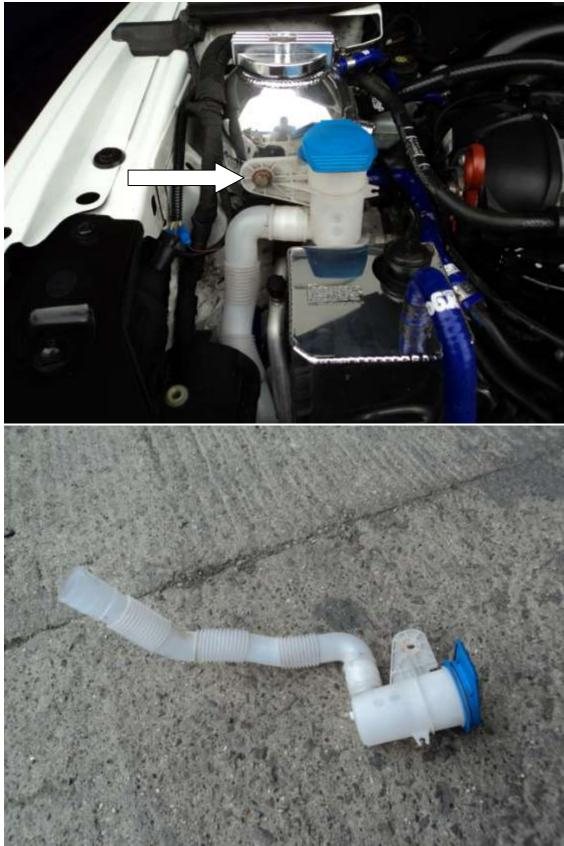
Fit the silicon 45 degree pipe on to the top of the washer tank and tighten with a hose clamp driver. Then fit the new forge washer bottle to the other end of the pipe, again securing with a hose clamp and tighten.
