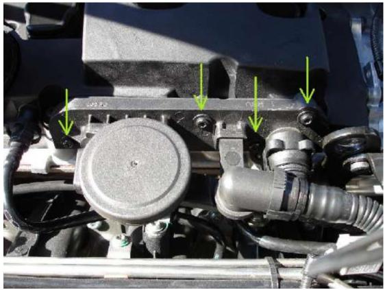
5. Remove any excess oil on the orange o-ring using a cloth. Fit the new Black anodized Forge PCV bypass plate using the screws you removed in the step above. Reattach the previously disconnected clip connector into the far right hand connection on the forge plate until the clip looks firmly in place.
