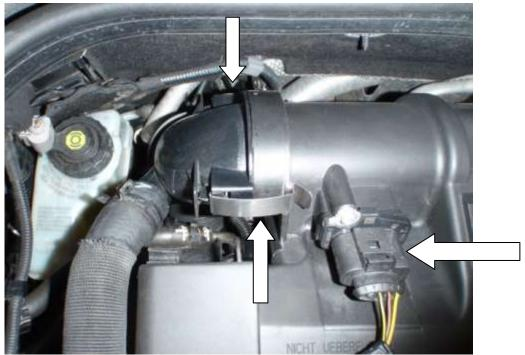
2. Unclip the connectors for both ends of the corrugated plastic pipe that connects to the PCV valve and intake manifold by squeezing the knurled clips at the end of each hose and simply pull out the hose.
