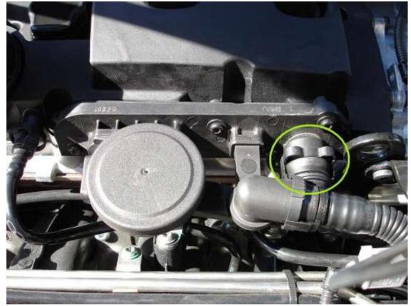
4. Using the T25 Torx bit, remove the 4 torx screws securing the PCV assembly to the valve cover. Now remove the PVC assembly from the engine.
