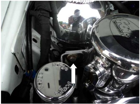
9. With the catch can in place, connect the 2 pipes from both catch can outlets to the PVC bypass plate. It doesn't matter which way round the pipes attach to. Secure with the cable ties supplied. If the hoses are too long simply cut off the excess.
