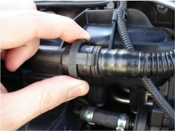
3. Very carefully using a flat headed screwdriver, unclip the connector on the far right of the PVC assembly. This connector secures at the top, bottom and both sides, so all 4 clips must be undone.
