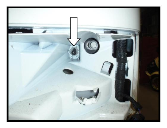
13. Pull out the wiring from the bottom and unclip it from the bumper on both sides.
