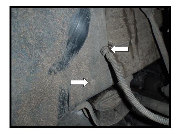
9. Remove the three T30 screws at the bottom of the bumper.
