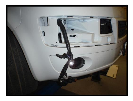
14. On the right side of the vehicle, unplug the connector from behind the headlight.
