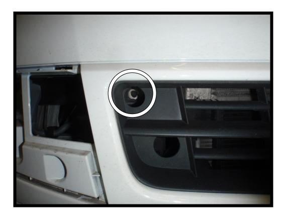
16. You will need to rest the bumper on some boxes or trestles, remove the front right light which allows clearance to remove the wiring. The bumper can now be completely removed.
