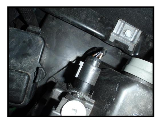
15. Finally remove the last two T30 screws behind the central moulding to release the bumper, and remove it from the car.
