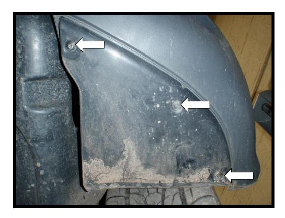
8. Undo the T25 screw and unclip the wiring in the inside of the arch liner.
