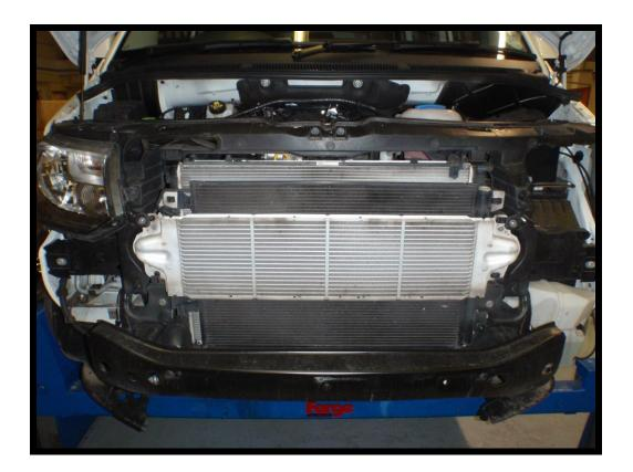
17. Remove the two T30 screws securing the intercooler to the chassis
