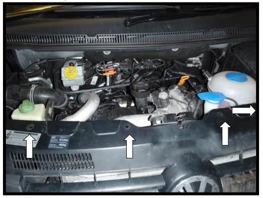
3. Pull the bottom of the grille forwards releasing the clips until the grille can be removed.
