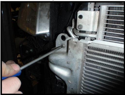
18. Using a screwdriver, lever the clips up that hold the hoses in the intercooler until they 'click' into their open position. You can then lift the intercooler off the hanging brackets and pull the hoses out of the back of the core to remove it from the vehicle.
