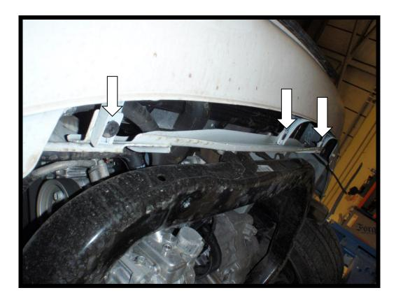
10. Now pull the arch liner away from the inner wing to expose the two 10mm nyloc nuts that need to be removed and the single T25 screw.
