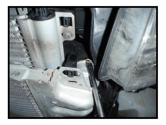
19. Remove the hose retaining clips from the stock intercooler and place them on the Forge intercooler in the same orientation. Place the Forge core on the vehicle and push the hoses in until they click into the retaining clips. Reuse the T30 screws to attach the Forge core.
