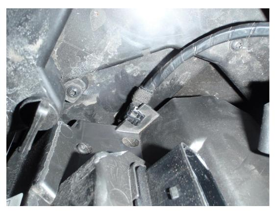
11. Finally remove the last two T30 screws behind the central moulding to release the bumper, and remove it from the car.
