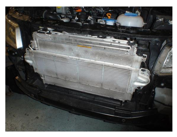
12. Remove the two T30 screws securing the intercooler to the chassis
