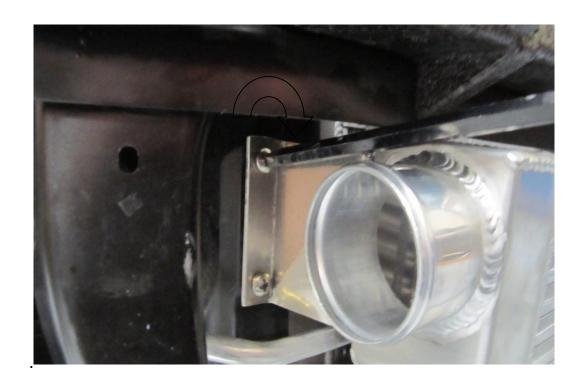
16.Place the temperature sensor removed in section 12 into the twintercooler as pictured
