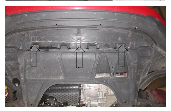
4. Pull down the arch liner, using your T25 Torx drive undo the fastener that attaches the bumper to the front wing .Then undo the two plastic nuts either side with your 10mm socket .As shown in the next picture.
