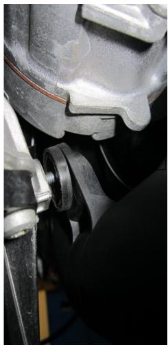
21.Once the hoses are in position tighten the jubilee clips then tighten the fasteners you removed from the lower boost pipe.
