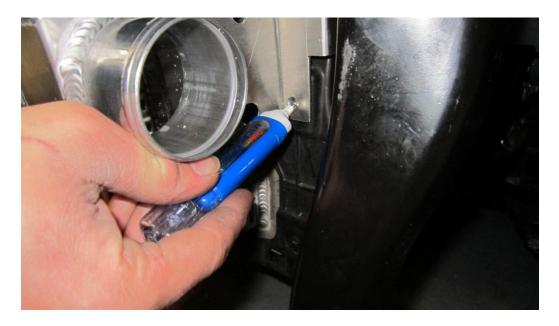
14. Using your drill make 4 holes in the plastic radiator cowling make sure these are in the correct position. Double check your twintercooler lines up, and is in the centre of the upper and lower crash bar before drilling.
