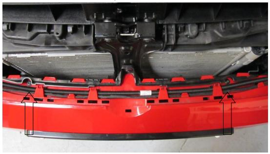
7. Now moving back to the sides of the car where the wing meets the bumper, pull towards yourself sharply to release the clips on the sides.
