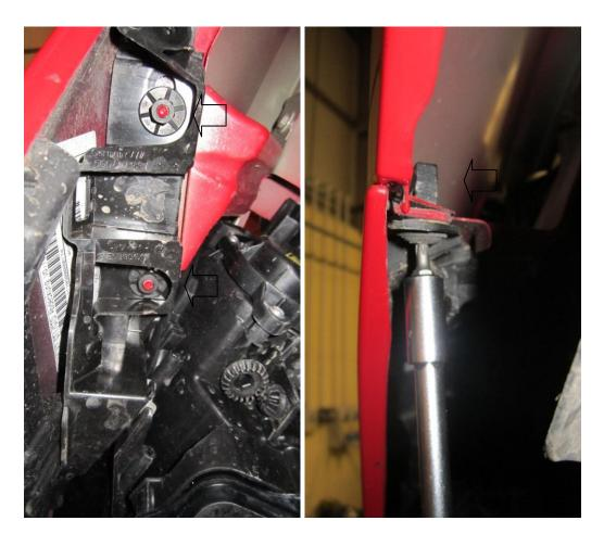
5. Using your T25 Torx drive remove the fasteners holding the grill onto the car. Once these are removed pull the grill towards you in a upward motion.
