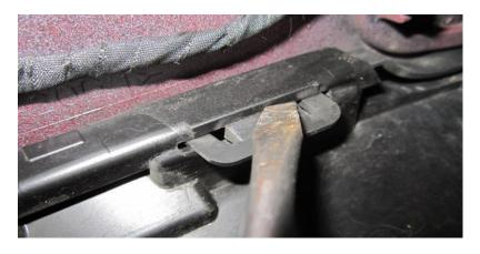
11. Remove the ducting either side of the condenser again using a flat bladed screwdriver .
