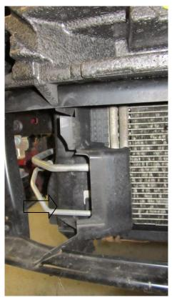
12. Disconect this temperature sensor on the lower side of the crash bar and bend the braket backwards. You will put this sensor on the mounting plate of your new Twintercooler once installed.
