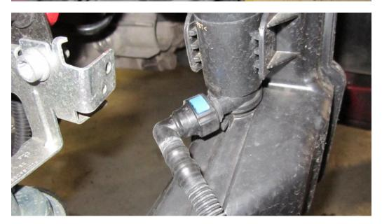
9. Once the bumper is removed the two plastic ducts either side need removed in order to make space for your new twintercooler.
