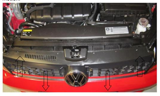
6. Now that your grill has been removed locate the two Torx T25 fasteners that hold the front of the bumper and remove .
