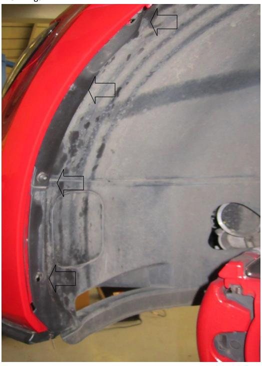
3. Again using your T25 Torx drive remove the fasteners from the undertray. This undertray can now be removed .
