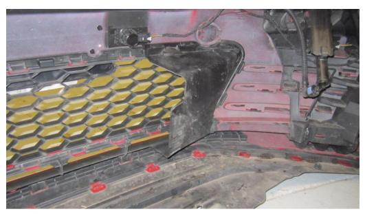
10. With a flat headed screwdriver press down on the clips to remove ducts.
