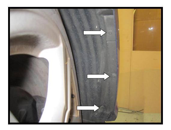
2. Undo all the t25 torx on the under tray and remove, undo and remove the t25 torx from the bumper.
