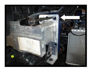
19. Undo the t30 torx on the radiator pack that will enable you to push back the radiator.
