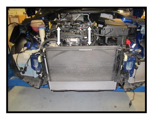
22. Once the radiator pack has been removed the remaining radiator and air condenser can be supported with a jack.
