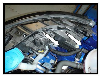
14. Remove the rubber ducting from the air filter.
