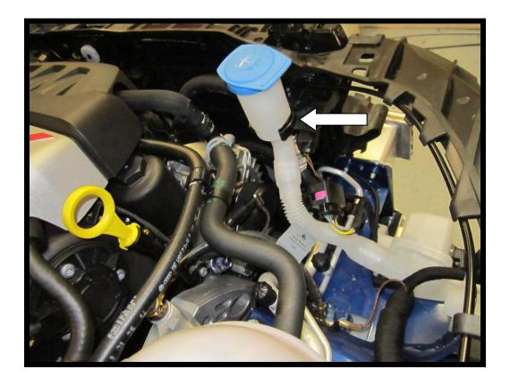
12. Unclip the plug next to the washer bottle and the same the opposite side. Under the washer bottle there is another plug on the radiator, this will also need to be unclipped.
