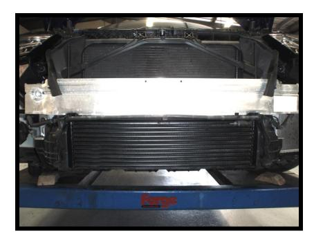
25. Making sure the intercooler is level with the radiator and crash bar, use a 6mm drill bit to drill a hole all the way through the bracket on the end tank and the rad pack. Using the nut bolt and washers supplied in the kit, secure the intercooler in position.
