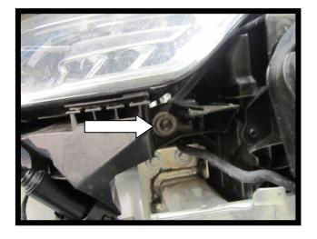
10. Remove the lights by undoing wiring loom, then remove the three t30 torx bolts two on top of the light and one behind. You will notice another two t25 torx as shown below. Undo these until the brackets are loose enough to remove the light.
