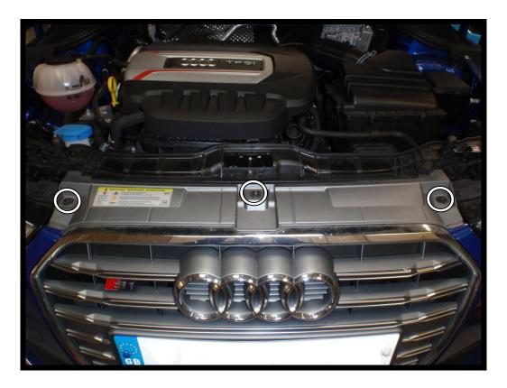
5. Remove the secondary radiator ducting by pushing it to the right until the clip is free.
