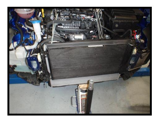
23. Trim off the small lip on the radiator cover. Placing the forge intercooler in the radiator pack will help you see the lip which hits the front of the intercooler end tanks.
