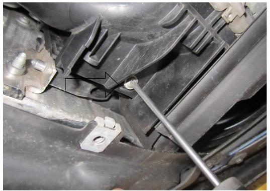
**6.** Pull the intercooler downwards to remove.
