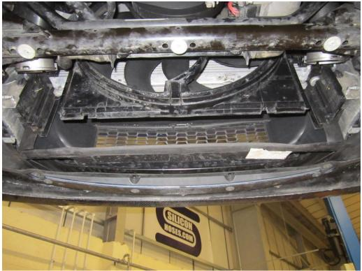
**7.** Place your new Forge Motorsport intercooler into position, making sure the tabs sit over your fan cowling. Connect your boost pipe couplers and use T25 fasteners to hold your new intercooler in place.
