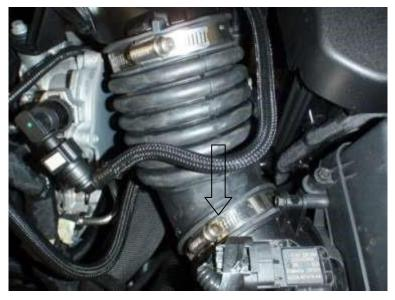
5. Unclip the the rubber cover that joins the air intake to the front of the car.
