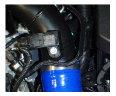
18. Using the 90deg. Silicone bend join the 76mm opening to the hard pipe and secure with the provided clip.
