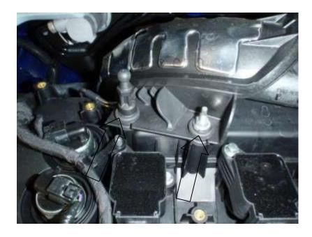
9. Using a hose clamp driver or similar tool undo the central jubilee clip.
