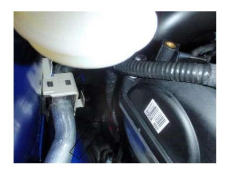
15. Place your Forge Induction pipe in position, connect the 19mm outlet to the open end of the silicone hose running from the cam cover, secure with a 25mm JCS clip. Bolt in place using the fixings provided.
