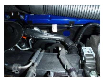
12. Using an 8mm socket undo the MAF sensor bolt and remove sensor from the standard air box.
