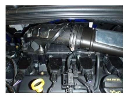
10. Undo the 8mm bolt on the second hard pipe and unplug the engine breather pipe from the back of the induction pipe.
