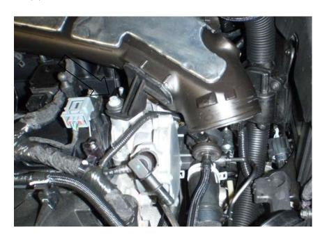
11. Unplug the standard engine breather pipe from the back of the cam cover.
