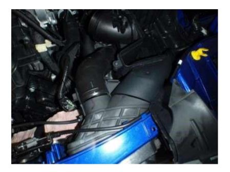
6. With a firm pull upwards release the standard air box from its rubber mounts.
