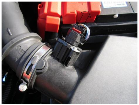
3. Using a flat bladed screwdriver pry the duct over the locater on the slam panel.
