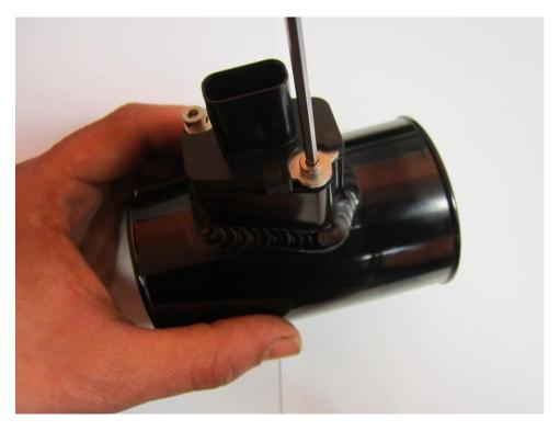
**10**. Now fit the MAF housing into the induction pipe making sure it is the same orientation as pictured.
