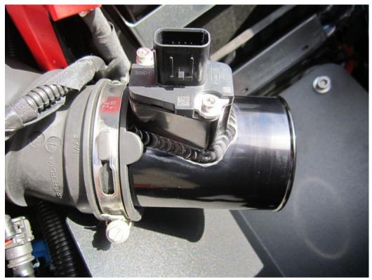
Now using your hose clamp driver fit the new high flow forge motorsport filter on to the end of the MAF housing .
