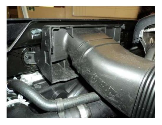
3. Unclip the flexible hose, pull off breather and remove. Unclip the cold air feed by pushing in the sides, Then pull out and remove. Undo the T30 screw and pull up the air filter box until it comes out of the rubber grommets and remove.
