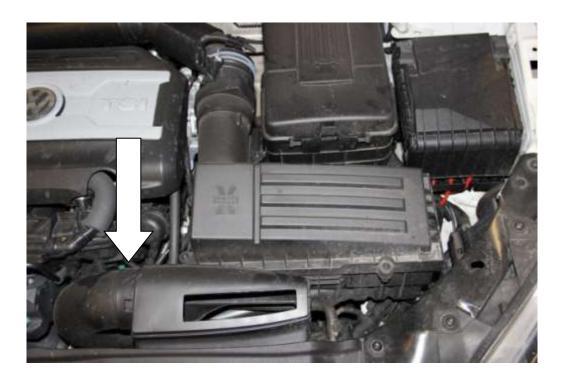
2. Using a hose clamp removal tool or suitable grips/pliers undo and remove the two hose clamps and remove the pipe.
