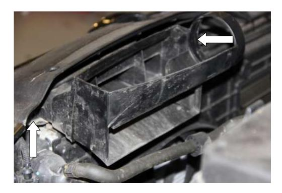
6. Undo the T30 torx bolt holding the intake pipe to the heat shield.
