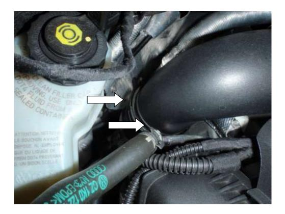
9. Now place the forge silicon hose joiner, two jubilee clamps and the new 90 degree aluminium pipe in place of the pipe you removed above. Then refit the breather pipe by pushing it on to the aluminium pipe.
