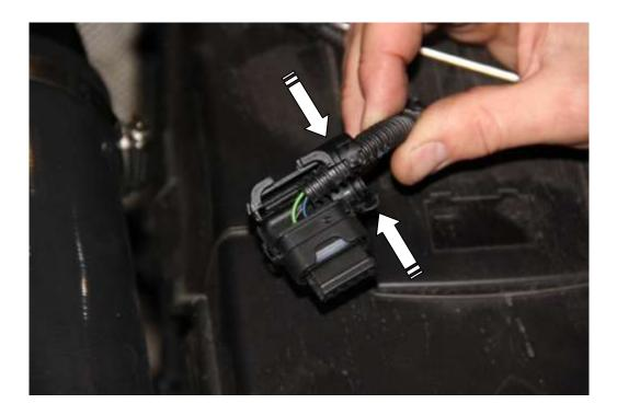
14. Fit the new silicon hoses along with the air flow sensor in the orientation shown below. Once this is done plug in the wire to the air flow sensor. (Please make sure when fitting the air flow sensor you have the arrow on the housing facing the same way as shown below).
