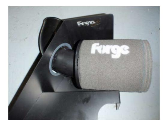
16. Install the cold air feed into position tighten the jubilee clip on the last silicon hose, and use the stock torx screws to fix to front of slam panel.
