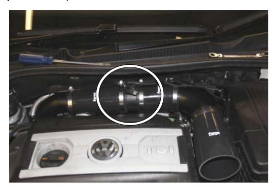
15. Fit the rubber trim and insert the filter into the cold air feed box.
