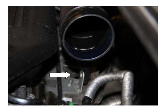
7. Squeeze the two breather tabs together to release the breather pipe from the intake.
