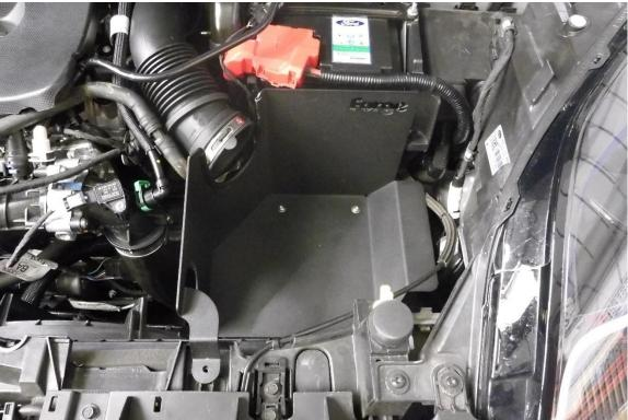
5. Using a 8mm socket and ratchet or pozi drive screwdriver secure the Forge Motorsport machined MAF tube into the the Forge Motorsport filter.
