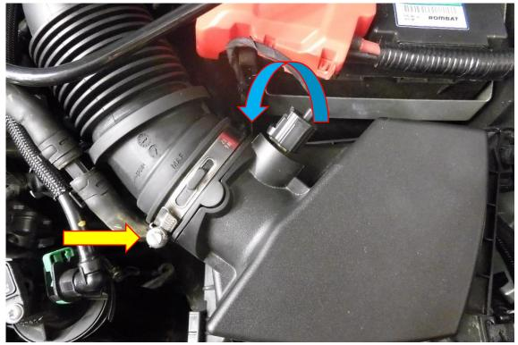
4. Fit the Forge Motorsport air filter tray into the engine bay, make sure both mounting pegs on the try locate into the OE rubber grommets.
