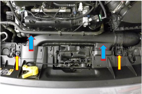
2. Move the coolant hose which is attached to the intake ducting. Push in both retaining tabs attaching the intake ducting to the airbox, this will then allow you to remove the intake ducting from situ.
