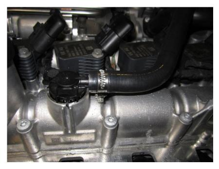
7. You can now tighten the final hose clamp that connects your silicon hose to the plastic turbo inlet hose. AGAIN TAKE CARE TO NOT OVERTIGHTEN THE HOSE CLAMP AS YOU COULD CRACK THE PLASTIC.
