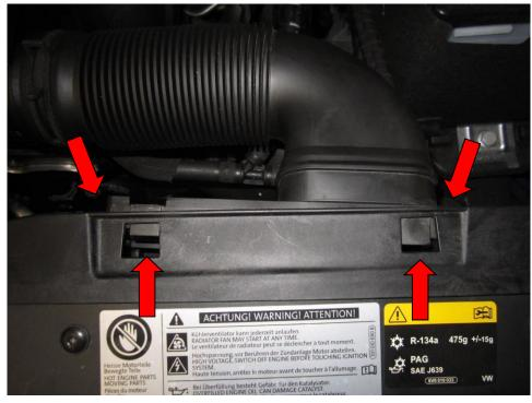
3. Remove the pipe from the airbox to the cam cover breather.
