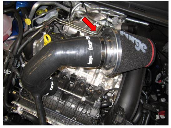
6. Fit the new silicon inlet hose into postion and connect the breather pipe to the rocker cover, then tighten the hose clamp.
