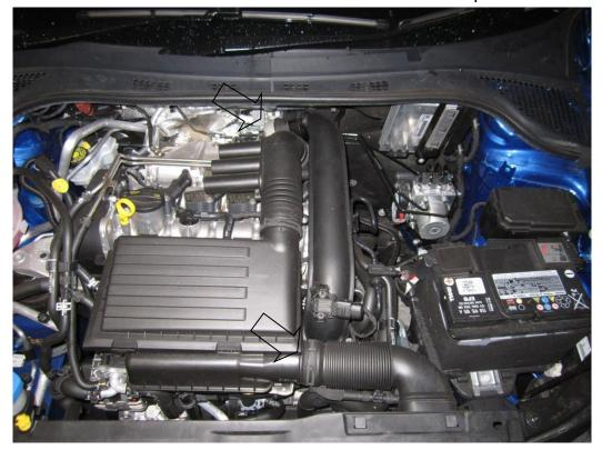
2. Now remove the inlet hose from its position by pushing down on the retaining clips as pictured below.
