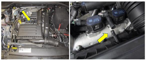
4. Remove the hose clamp that holds the airbox to the turbo inlet hose.
