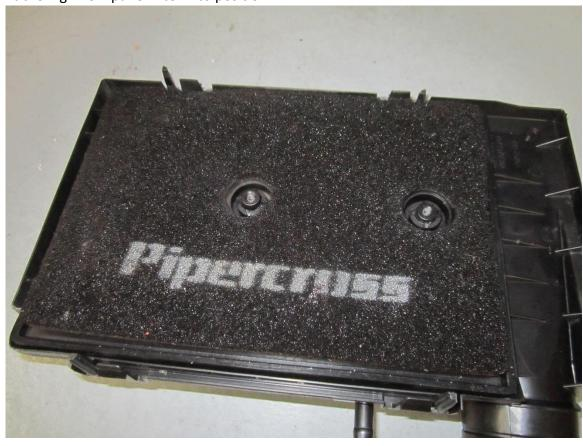
**11.** Attach the new carbon fibre high flow lid onto the OEM airbox lower half using the original fixings.
