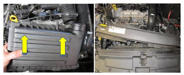
**6.** Using a T25 Torx Drive remove the two fasteners that hold the turbo inlet pipe in position.
