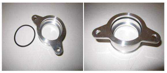
8. Using the M6 Allen caps bolts provided fit the turbo adaptor into position with a 5mm Allen key.
