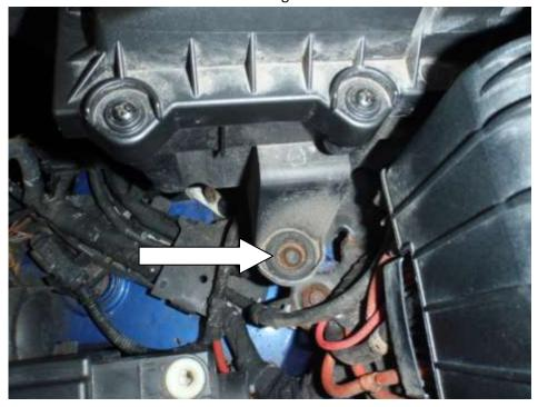
7. Undo the 3 bolts connecting the air box bracket to the car and remove.
