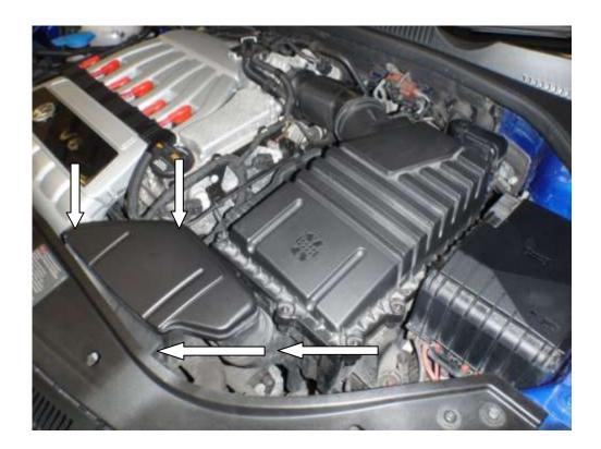
2. Remove the air intake scoop using a T25 torx screwdriver
