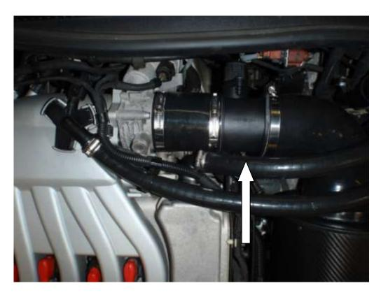
10. Fit the new air scoop using the original screws
