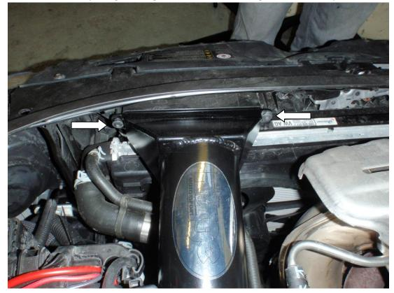
7. Attach both ends of the cold air pipe to the cold air scoop and air filter using the hose clamps supplied.
