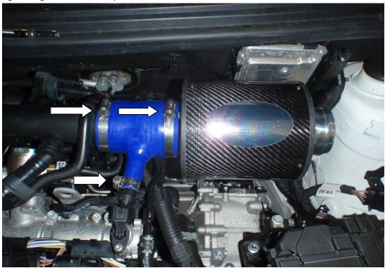
6. Fit the cold air scoop using exsisting T25 screws from the original cold air scoop
