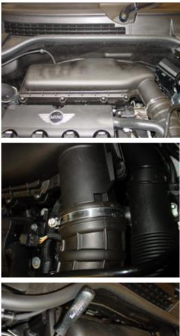
At the rear of the engine the Air Box is located.
