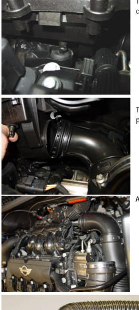
The airbox is secured by plastic pins that locate into rubbers. The airbox can be gently pulled upwards in order to dislocate these.
