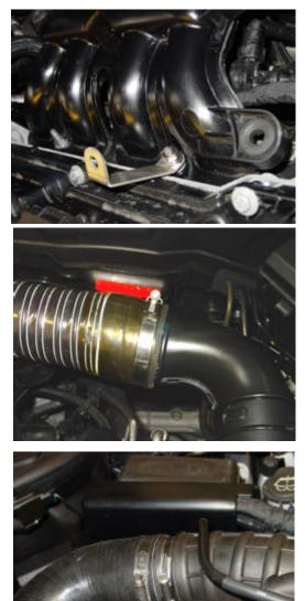
The bracket that will secure the new induction kit is fixed to the intake manifold stud using the 13mm locknut.
