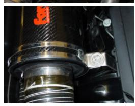
The carbon canister / filter housing is secured to the previously fitted bracket with the M8 x 25mm hex bolt and Nyloc nut. A washer is used between the bolt head and the canister bracket as shown.
