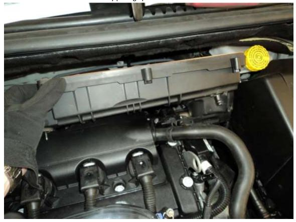
9. Using a 8mm socket and ratchet undo and remove the 8mm bolt holding the air flow sensor into the manifold. Then pull upwards on the sensor to remove it.
