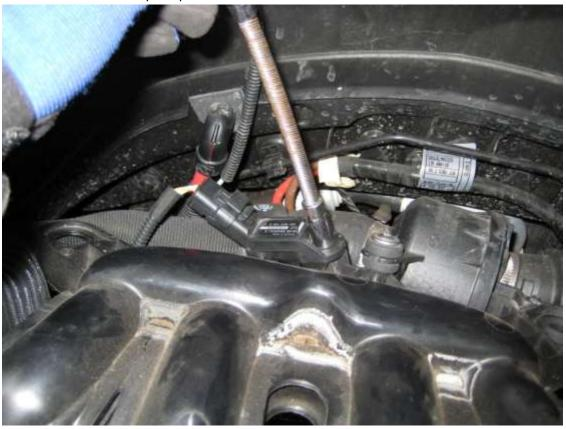
10. Fit the sensor to the aliminium vac block supplied, then fit the vac block to the inlet manifold using the philips screw provided.
