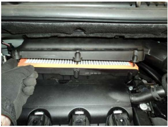
8. Remove the bottom of the air box by pulling upwards to realease it from its rubber mounts.
