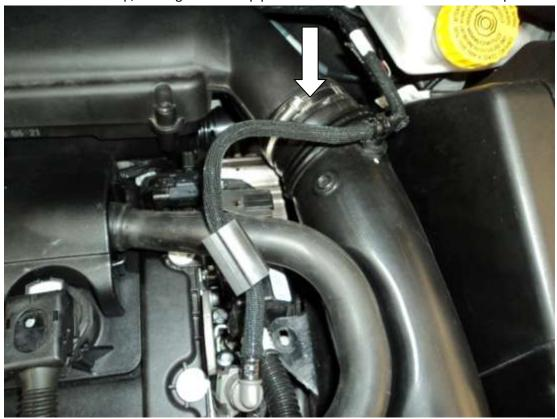
7. Undo the four T20 Torx holding the top of the air box to the bottom section. Then remove the top part of the air box.
