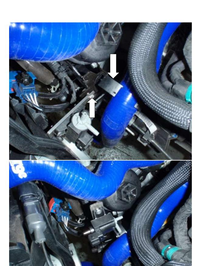
4. Use the wiring loom provided. You will need to trim the 2 small lugs on one end to make it fit into the oem plug.
