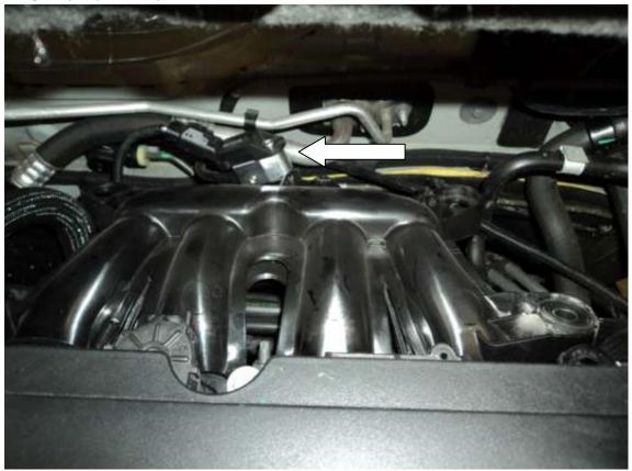
11. Using the vac tube provided cut to desired length to fit accordingly to the diagram below. Use the cable ties provided to secure the vac pipe and prevent it from fouling the cooling fan.
