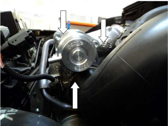
3. Using the hole that is situated on the lower coolant pipe bracket, fit the solenoid in place with the 10mm bolt, washer and nut provided. ( you may find this easier by undoing the plastic hose clip to give you more room).
