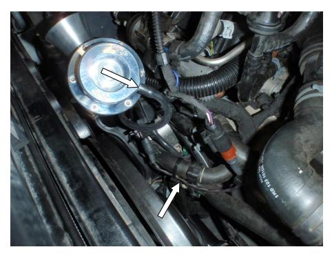
8. For venting to atmosphere at the back of the engine bay install the silicon hose, bung and clips supplied in the kit onto the filter pipe.
