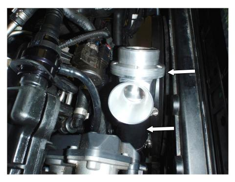
6. The photo below shows how to install the vacuum hoses and wiring extension. When installing in the car, the vacuum hoses and wiring extension can be routed under the inlet manifold for a neat installation.
