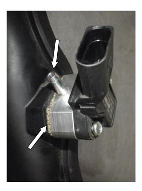
5. Install the silicon hose and BOV with the clips supplied in kit.
