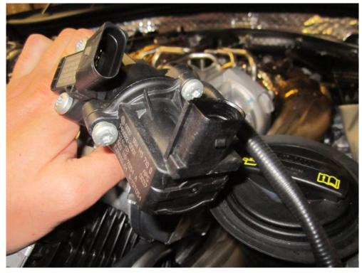
5.Before mounting the Forge Motorsport valves into position, ensure the o-rings supplied are pushed fully into the lower part of the valve. Failure to do this will stop the valve from working correctly.
