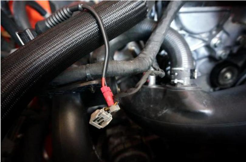
12. Now attach the forge loom to the solenoid.
