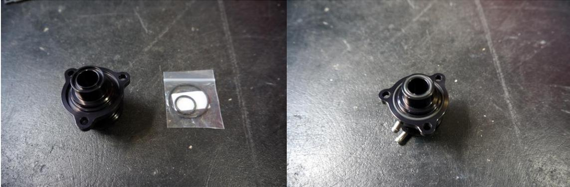
5. . It is easier if you assemble the solenoid before you attach the Forge valve to the charge pipe as pictured below.
