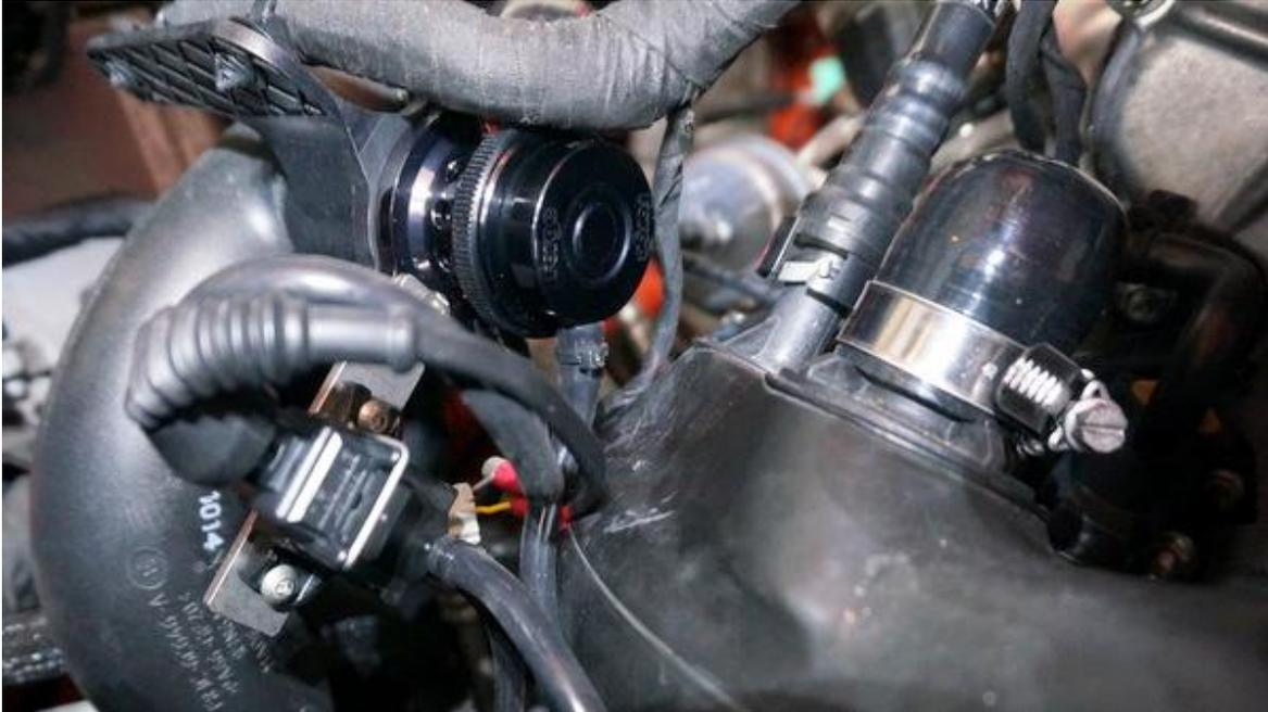
13. BEFORE STARTING THE VEHICLE DOUBLE CHECK THE CONFIGURATION ON THE WIRING LOOM AND VACCUM LINES TO THE SOLENOID.
