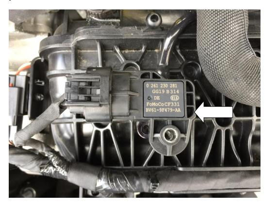
10. Fit the boost take off adapter supplied using the T25 torx screw. Fit the boost sensor using the supplied cap screw.
