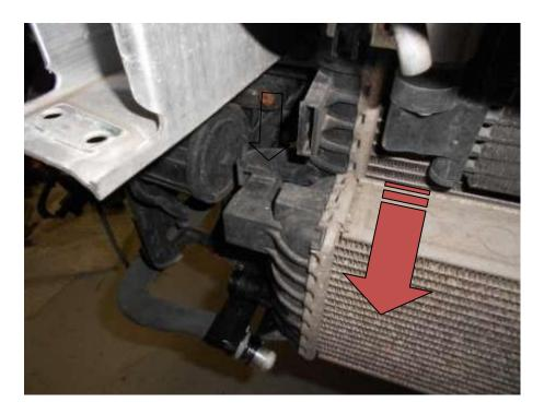
24. To allow better access to the pump and secondary radiator. Undo T30 screw and unclip hose clips.
