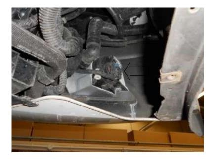
4. In each wheel arch undo 2x T30 Torxs screws.
