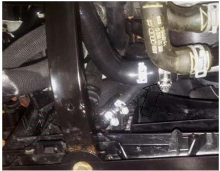
60. Using the remaining silicone hose connect I to the right-hand outlet of the chargecooler and connect J to the side inlet on the expansion tank and secure with a 2x suitable hose clamps.
