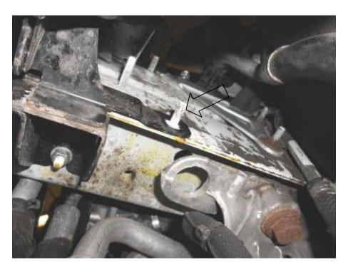
35. Using the silicone bung provided, place over the 16mm hardpipe and secure with a suitable clip.
