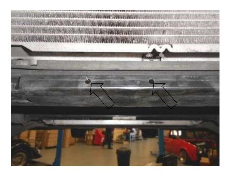
40. Using the 1x T30 Torx screw and M6 washer, bolt the oil cooler in position. Place an M6 Washer underneath the T30 Torx screw.
