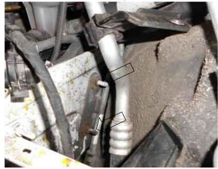
Undo 2x 10mm Nuts on the side of the chassis leg.
