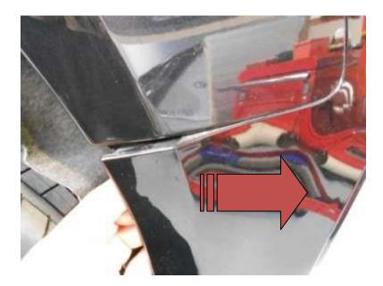
14. Using a flatblade screwdriver unclip x3 clips and remove crash bar cover.
