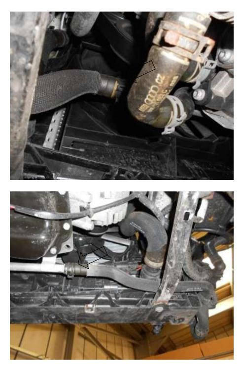
Undo 2x 10mm nuts and remove hardpipe and OEM chargecooler hose.
