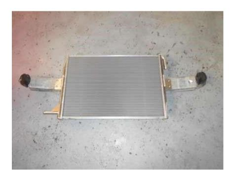
54. Using the 8x Posi-drive screws provided attach the chargecooler to the back of the crash bar.
