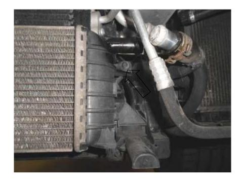
23. Unclip the left-hand end of the chargecooler and tip it forward to remove.
