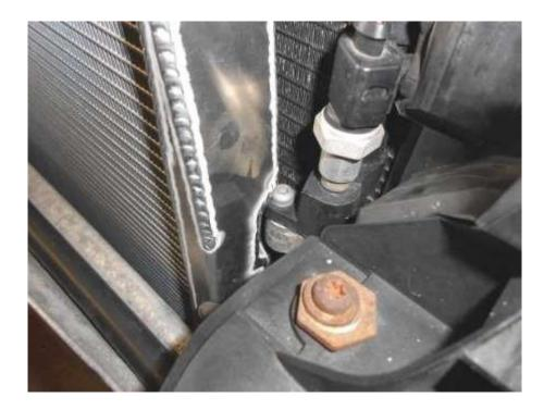
51. Remove the crash bar from the vehicle and place the chargecooler back in position.
