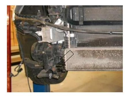
21. Using a suitable hose clamp removal tool disconnect the hose at the other end of the charge cooler.
