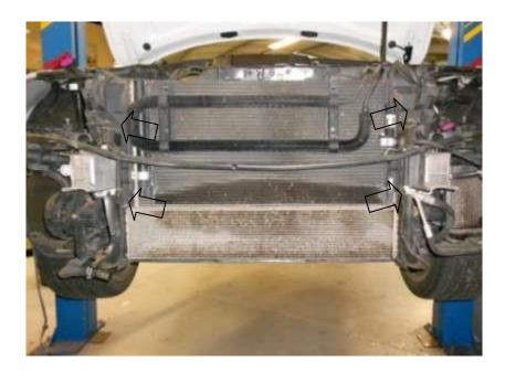
20. Drain coolant from the vehicle. Using a suitable hose clamp removal tool disconnect the lower chargecooler hose. Ensure that the vehicle has fully cooled down before attempting to drain and work on the coolant system. Failure to do so may result in damage to the vehicle or personal injury.
