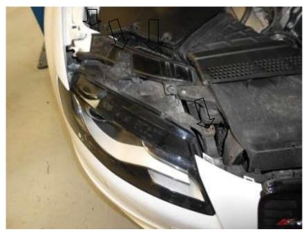
11. Using a 10mm spanner reach inside front wing and undo 1x bolt on both sides of the car.
