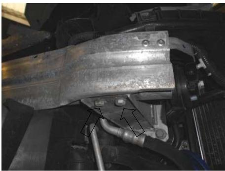
19. Unclip and remove both air-guides.
