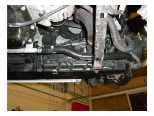
57. Using the custom silicone hose provided and 2x suitable clips connect **C** to the pump inlet and **D** bottom of the expansion tank.
