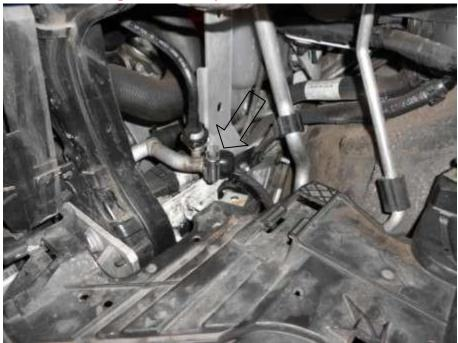
36. Using 2x M8x16mm socket cap bolts and 2x M8 washers secure the expansion tank to the bracket.
