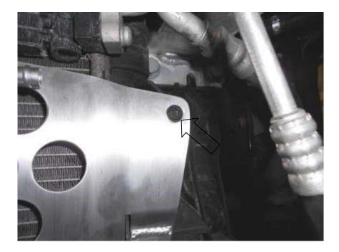
41. Using the 2x M6x16mm Allen cap bolts, 4x M6 washers and 2x M6 Nyloc nuts, secure the other end of the oil cooler.
