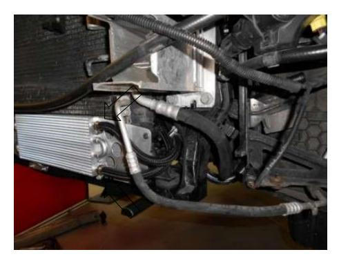
45. Cable tie rubber pipes to back of the fan shroud. Make sure the fan can still rotate freely.
