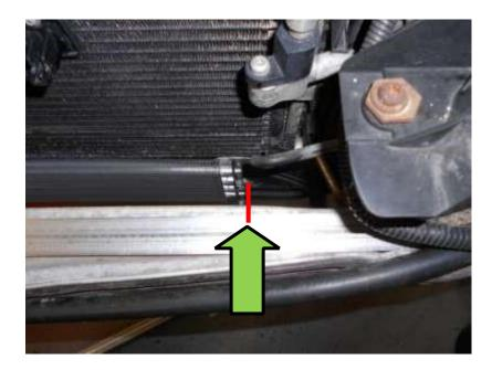
50. Carefully hold the chargecooler in position, check that nothing touches the A/C radiator or condenser.
