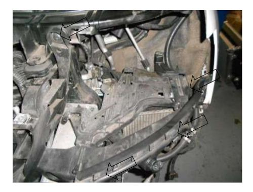
25. Pull the plastic part forward and from underneath undo the 2x T30 Torxs screws and remove the head light platform.
