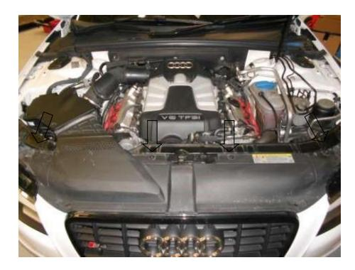
6. Push the 3x tabs down and carefully pull the front of the cover backwards to release it. Store in a safe place away from the vehicle to prevent damage during the rest of the installation.
