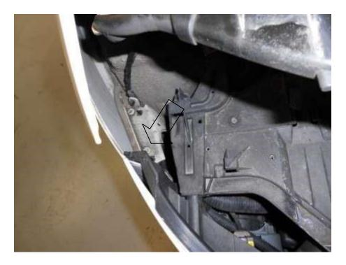
12. Undo X2 T25 Torxs screws on the top of the bumper.
