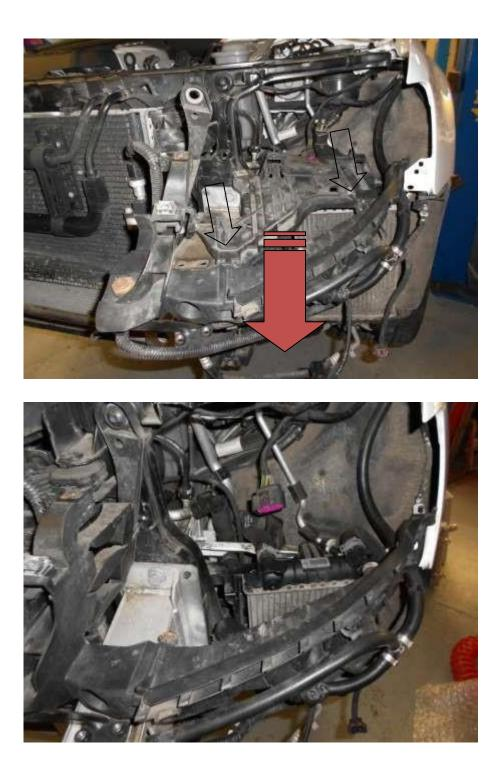
26. Inside the wheel arch remove 2x clips.
