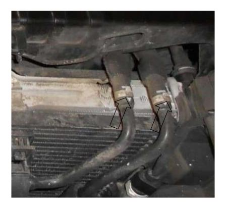
43. Carefully disconnect the pipes to the oil cooler, block with a suitable sized bolt (10mm Diameter).
