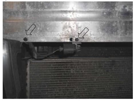
16. At each end of the crash bar unplug both horns and unclip the cable clips.
