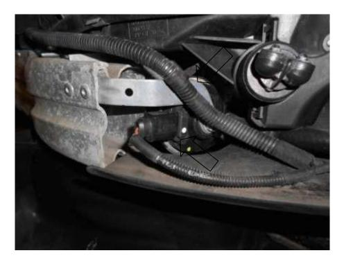
17. Unclip the secondary radiator ducting and remove it from the vehicle.
