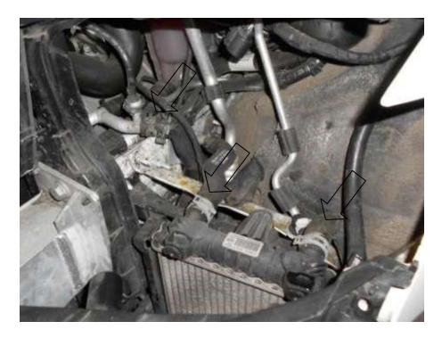
28. Undo the 2x T25 screws and lift the secondary radiator upwards to remove it. Store in a safe place away from the vehicle to prevent damage while working on the rest of the installation.
