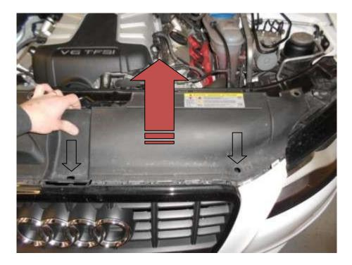
7. Undo 2x T25 Torxs screw and unclip the air intake from the airbox.
