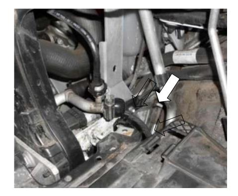
34. Using 10mm spanner replace OEM nut on the side of the chassis leg.
