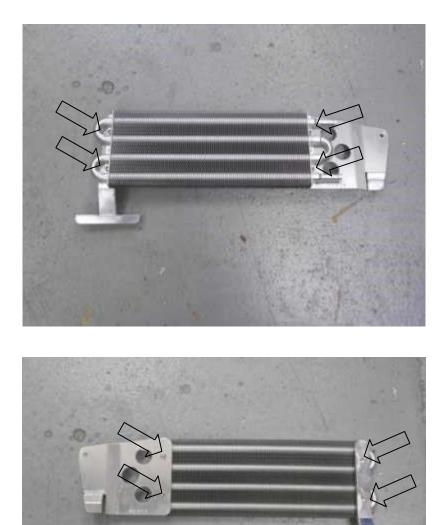
39. Place the oil cooler in position on the car. Using a marker pen or similar, mark the hole positions for the bottom bracket. Remove the oil cooler from the car. Using a drill and 6mm drill bit drill both bolt holes for the bottom bracket.
