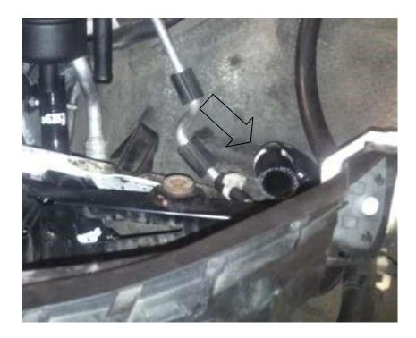
59. Using the silicone hose provided connect **H** to the open side of the outlet of the chargecooler pipework. Connect **G** to the left-hand outlet of the secondary radiator when it is refitted.
