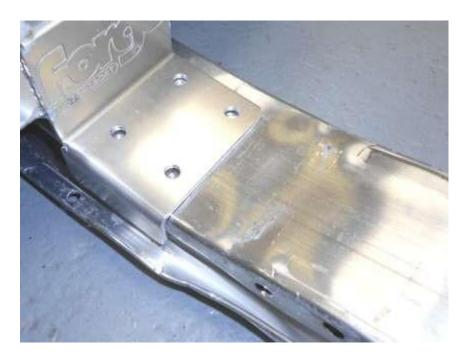
53. Using a drill and 5mm drill bit drill the 8x holes.
