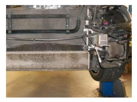
22. Undo T30 Torxs screw on right-hand side of chargecooler.
