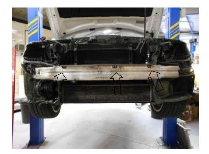
15. Using a flatblade screwdriver push the centre out of the clip and remove the sensor and cable clip.
