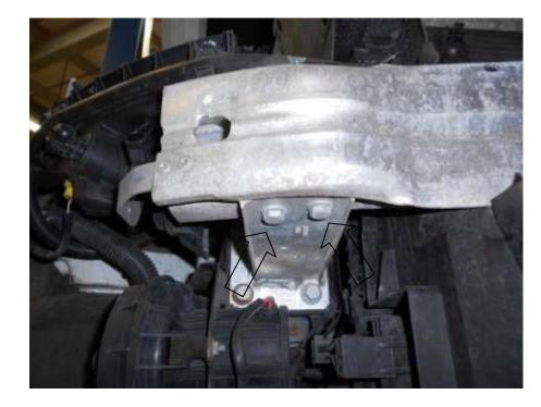
18. Using 13mm socket or spanner undo 2x bolts at each end of the crash bar. Pull the crash bar forward at each end to release it.
