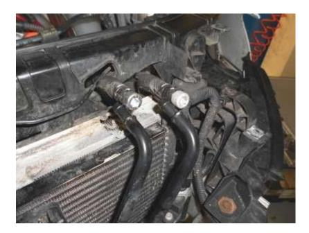
44. Using the 2x 285mm long hose extensions, hose joiners and suitable clips. Reroute the rubber pipes and join them to the new oil cooler.
