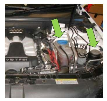
64. Top up the Forge expansion tank with coolant so the level is just above the baffle plate. After running the engine up to operating temperature (this may take 15-20mins) allow the car to cool before checking and topping up the coolant if required. Bleed air from the chargecooler coolant system by undoing 2x bleed screws shown below.
