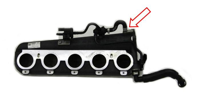
1. Remove the vacuum hose as indicated above, unscrew the vacuum pipe and screw in the new pipe with the washers and banjo take off.
