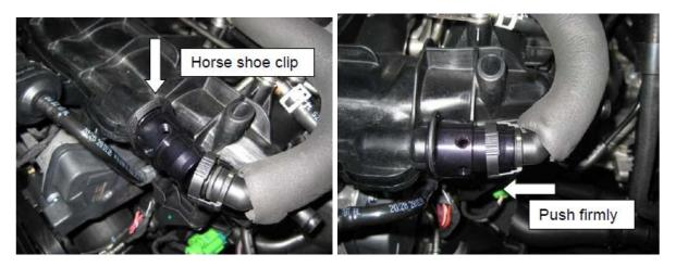
The Forge vacuum take-off adaptor is installed as shown. It is necessary to push the adaptor onto the spigot so that the retaining horse-shoe type clip can be slid into place fully (shown above with vacuum nipples removed for clarity).
