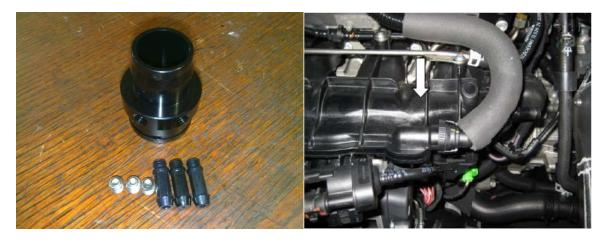
At the front right (transverse engines) you will see the OEM vacuum hose connector. By squeezing the sides of the OEM connector the locating clips are released so that the connector can be withdrawn.
