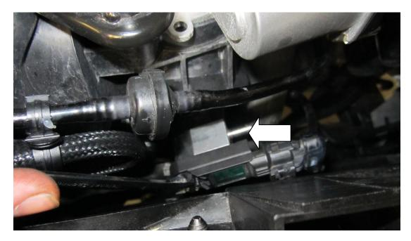
8. Now fit your forge dump valve. There are two different orientations depending on your application; if using the forge atmo valve you will need to fit the 25mm blanking plug and silicon tube provided.
