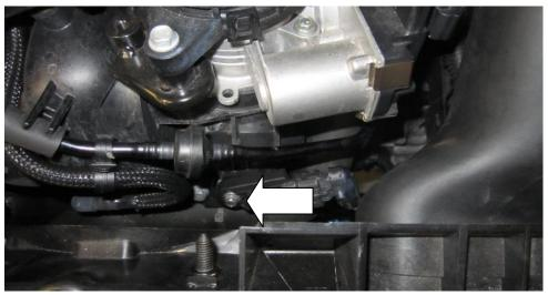
7. Fit your boost and vacuum take-off block and refit your sensor using the new longer fastener provided .
