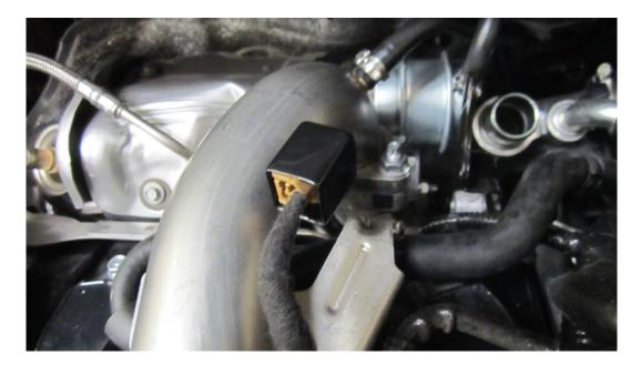
12.If your valve is the recirculating type connect the silicon pipe to where it has been blanked in step 10.
