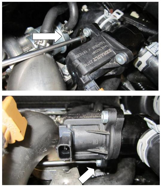
4. Using your hose clamp driver remove the two hose clamps that keep your valve attached to the induction pipe and turbo inlet.
