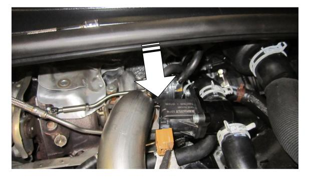
3. Using your T27 torx drive remove the two fasteners that hold the value in place
