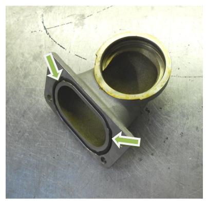
9. Test fit the cast elbow and boost tap without bolts to correctly align the holes in the cast elbow and billet boost tap.
