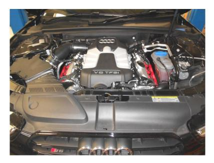
2. At the back on the engine carefully pull the plastic cover upwards.
