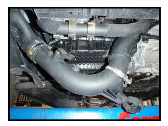
5. Fit the forge silicon hose so that the dump valve extension fits between the radiator and inlet manifold. Reattach the plastic boost pipe. Move the silicon hose around until it fits in the correct position and tighten the hose clips.
