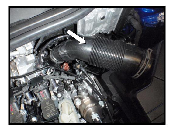
8. Unplug the wiring and remove the OEM dump valve
