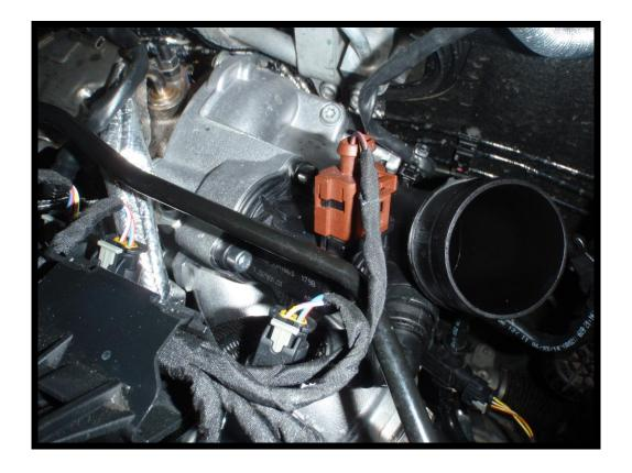
9. Bolt the forge solenoid next to the vacuum pump as shown below. Connect the OEM dump valve wiring to the forge wiring loom and plug into the forge solenoid.
