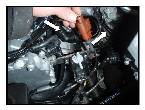
10. Install the dump valve blanking plate/boost take off plate to the turbo. Cut through the vacuum pipe and add the T-piece, then connect the hoses as shown below.
