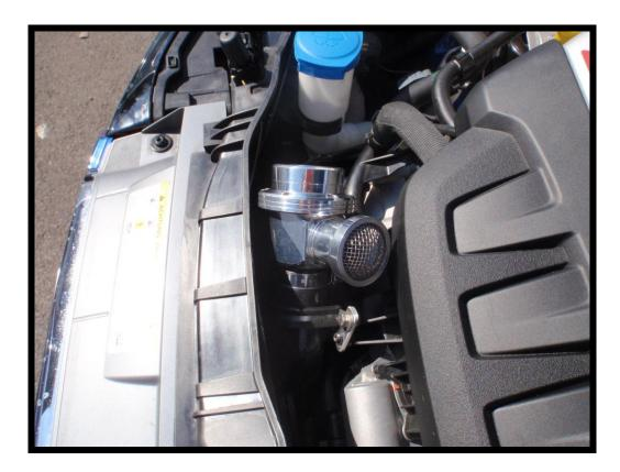
6. Fit the dump valve with hose clip and P-clip using the small bracket and bolt supplied in the kit. Attach to the inlet manifold and tighten using the screw previously removed.
