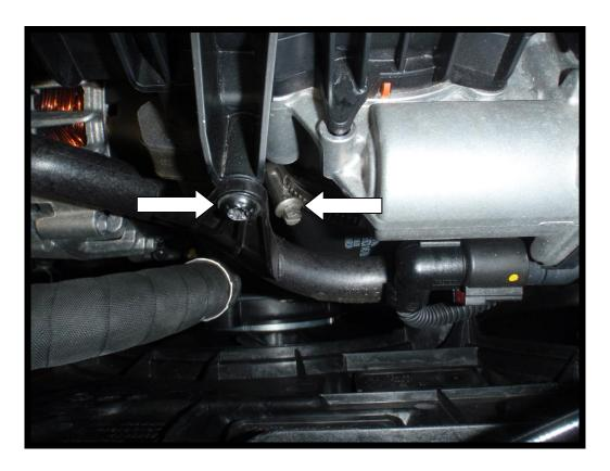
2. Jack up the car and support on axle stands then remove the under tray using a T25 torx
