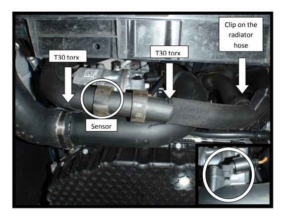
4. Undo the bottom hose clip, pull the plastic boost pipe down and remove the hose connected to the throttle.
