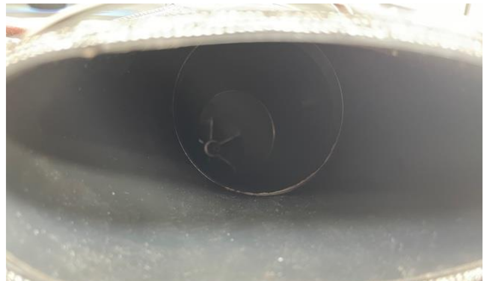
24. Make sure the silicon is fully pushed onto the inlet. The internal step of the silicon should be flush against the inlet.
