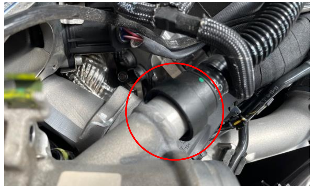
12. This breather attachment is secured with small internal clips. Use a small screwdriver or pick to push the clips back in order to release the tube from the inlet.
