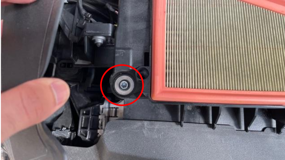
5. Unscrew the Torx screws on each side of the airbox.
