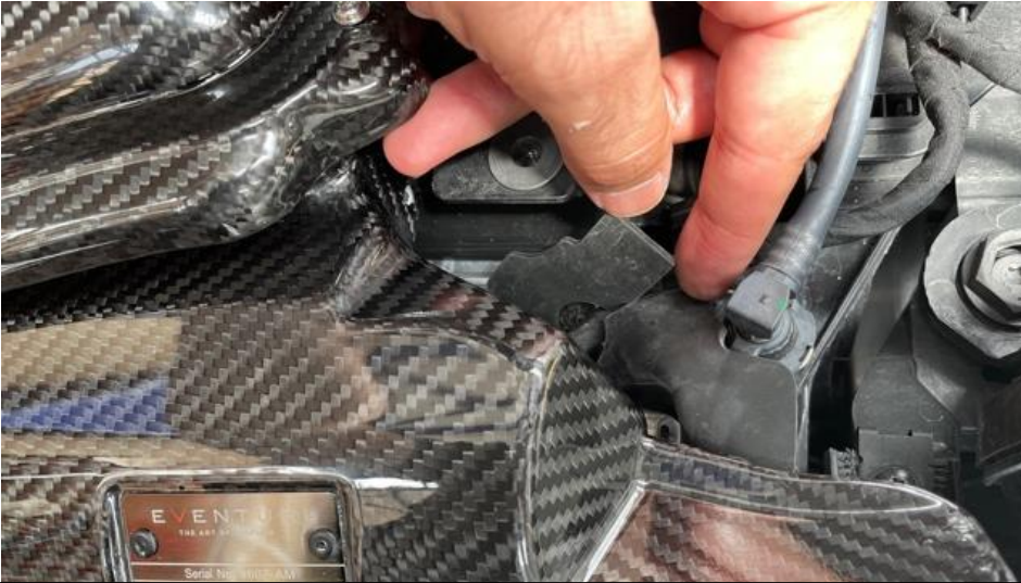
31. On both sides of the airbox there will be rubber flaps. Push these aside to give the airbox clearance to sit flat on the slam panel.
