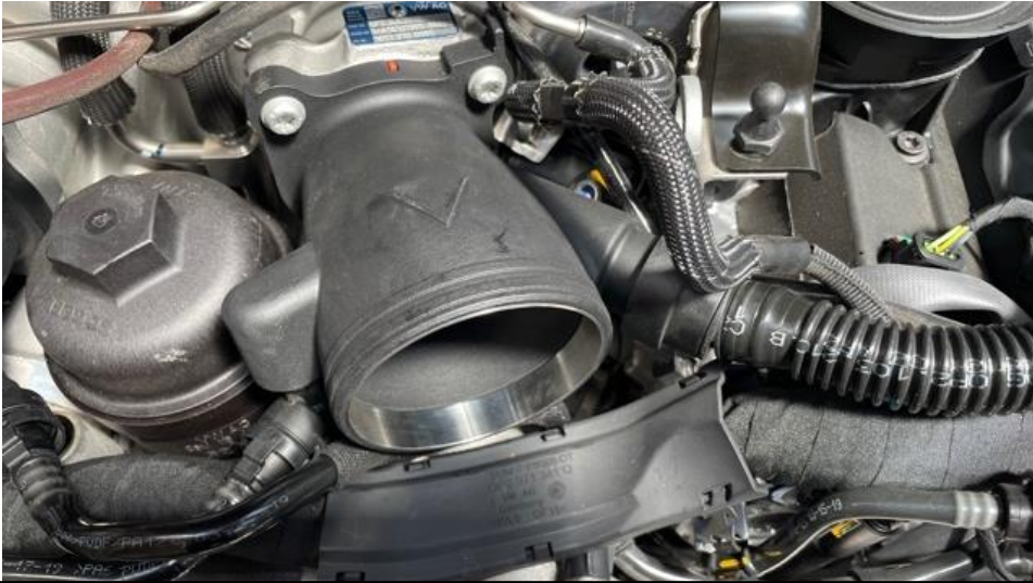
25. Repeat for the Right side inlet and also push the breather hose onto the inlet.
