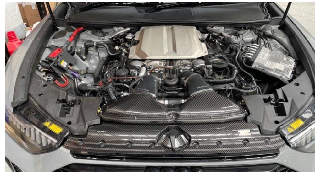
38. Install the side covers again. Once pushed back into the press clips they can also be hooked into the side brackets of the airbox.
