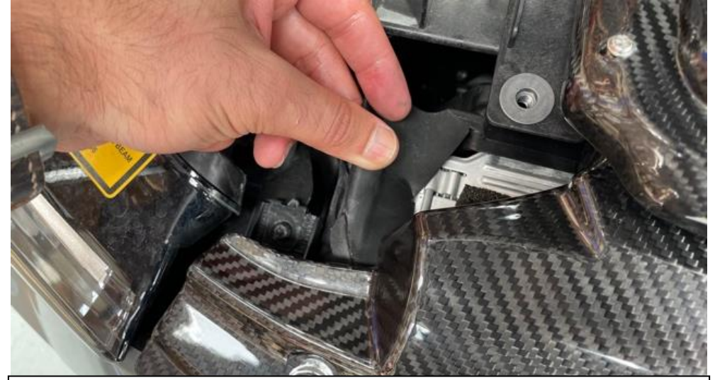
32. Rubber flap on the left side. Move away for clearance.
