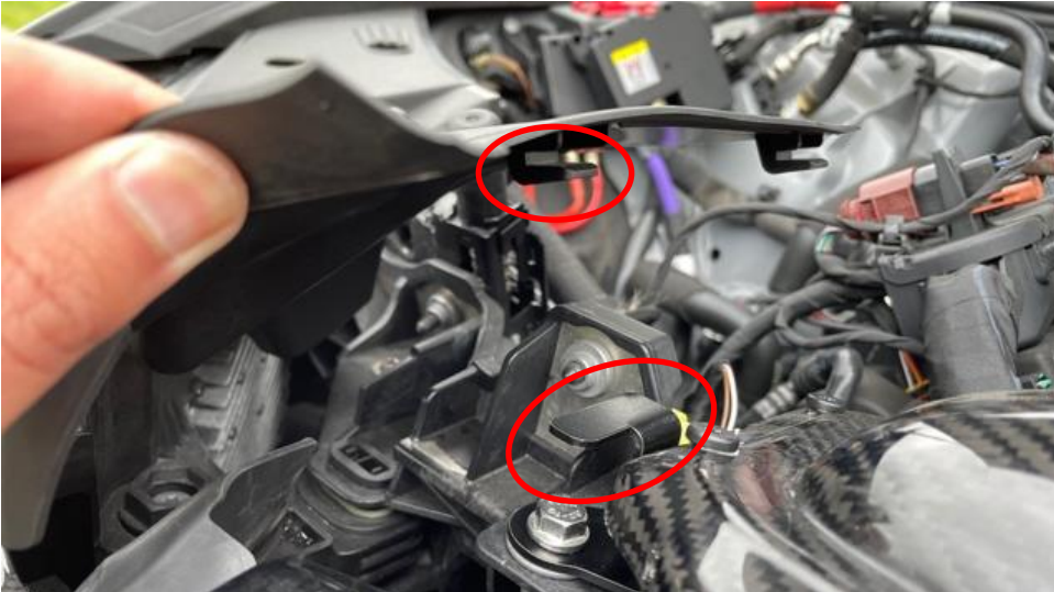
38b. The tabs on the side panels can be hooked into the brackets as shown.
