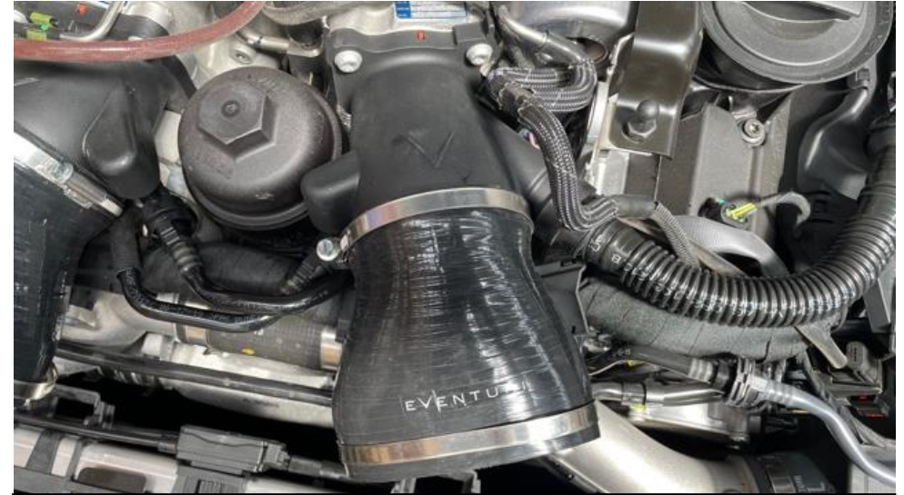
26. Push the second silicon hose onto the inlet. Position the clamps as shown and leave them loose.
