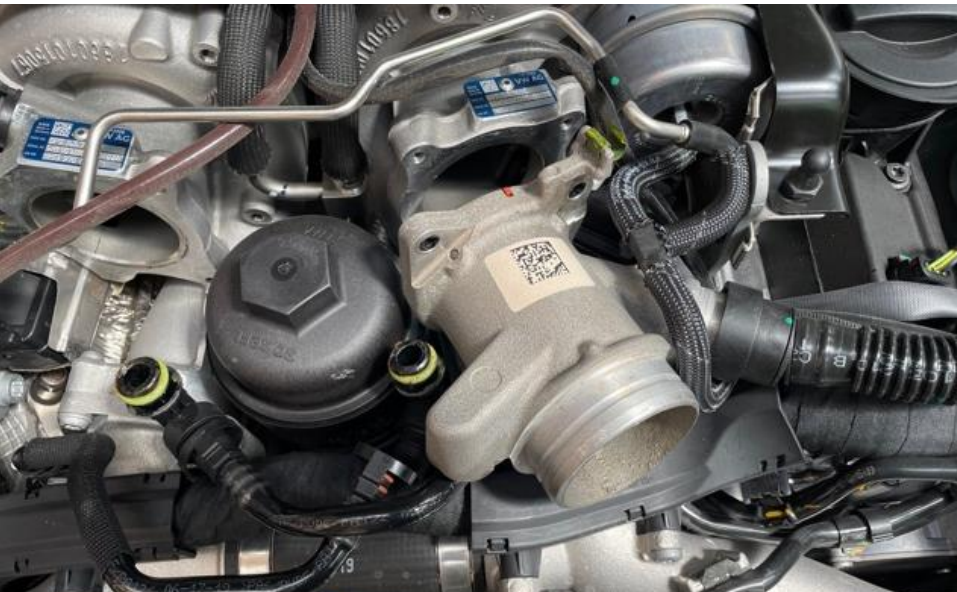
11. Remove the 3 Torx screws holding the right inlet in place. Remove the inlet and also remove the breather attachment - see next step.
