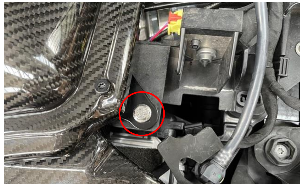
34. Using the supplied M6 bolts, secure the brackets on both sides. Bracket has been updated from the one shown.
