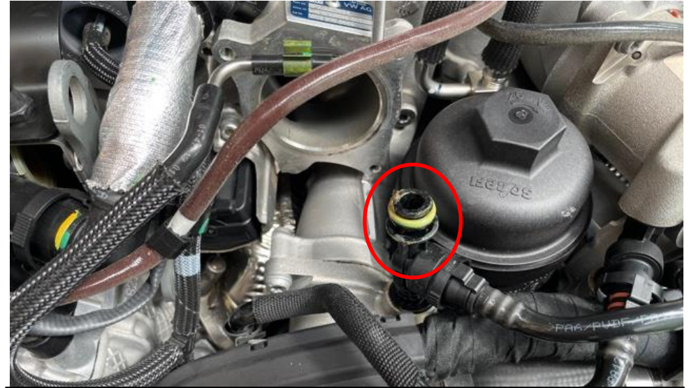
10. Remove the inlet. Note the breather which goes into the inlet also (circled).
