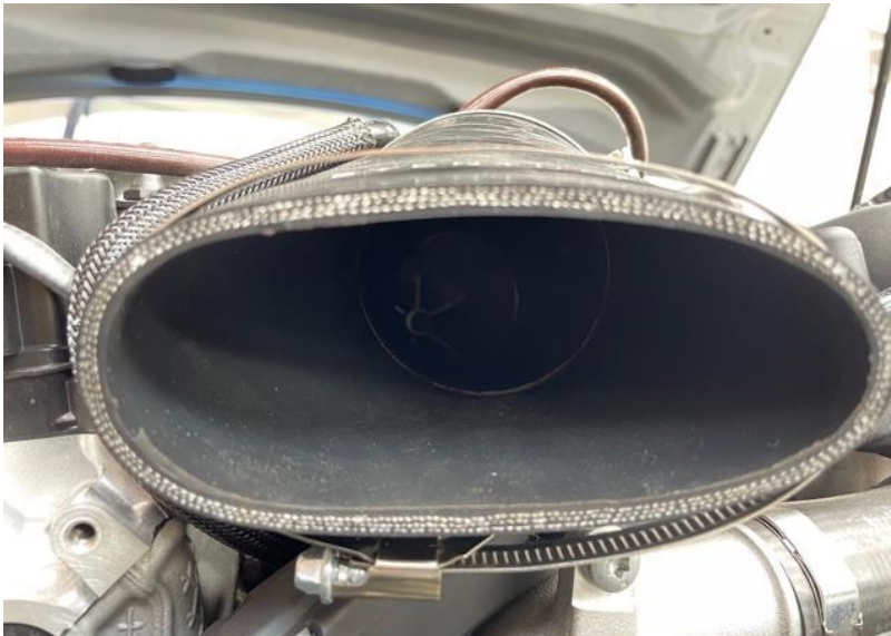
27. Position the lower clamp with the head underneath and directed towards the middle of the engine.
