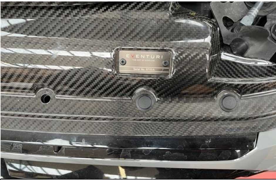
33. Insert the plastic push rivets into place. Make sure the airbox is fully down onto the slam panel.
