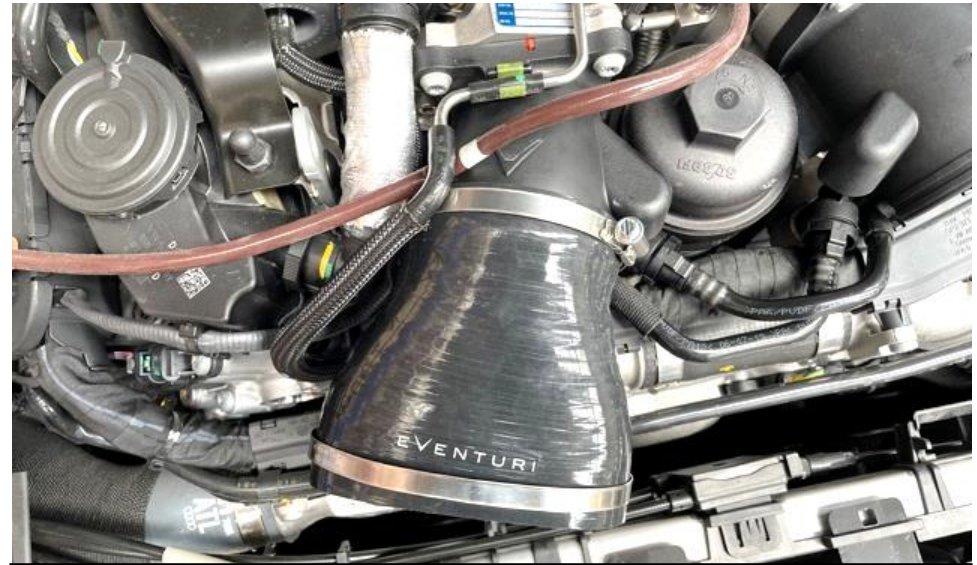
22. Push one of the silicon couplers onto the inlet with the hose clamps on both sides. Keep the clamps loose and position the heads of the clamps as shown.
