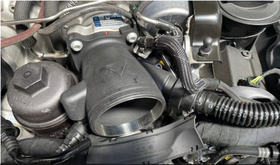
21. Secure the inlet with all 3 screws.
