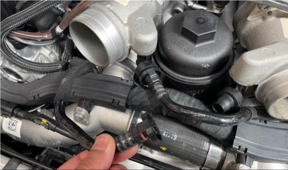
9. Unclip this breather and move it away to gain access to the lower torx screw.
