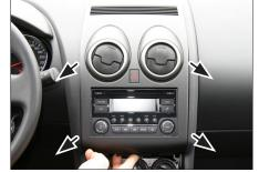
4. Unclip and remove OEM panel
