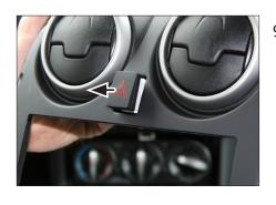
Remove hazard light switch from OEM panel
