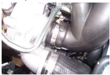
2) Remove the intake pipe at both ends and remove to gain access to the solenoid.
