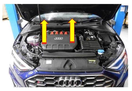
2. With the engine cover removed locate the original diverter valve. This is located on the boost pipe at the lower front of the engine.
