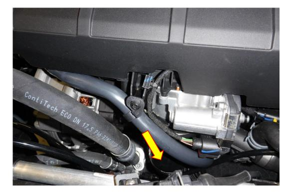
3. On the OE valve push back the red retaining clip to allow you to remove the wiring loom. Remove the three T25 Torx fasteners attaching the OE valve to the boost pipe, the OE valve will now come away.
