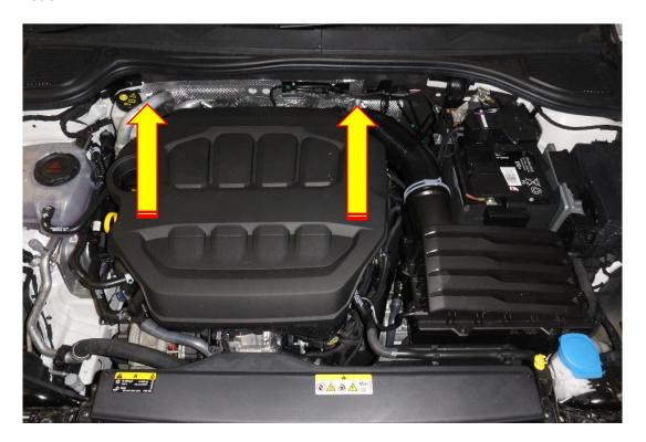
2. With the engine cover removed locate the original diverter valve.
