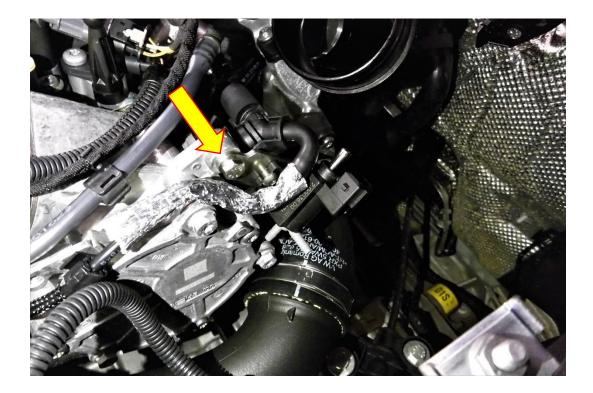
8. Take the wiring loom supplied in the kit and connect it to the solenoid and the other end to the loom which was attached to the OE valve.
