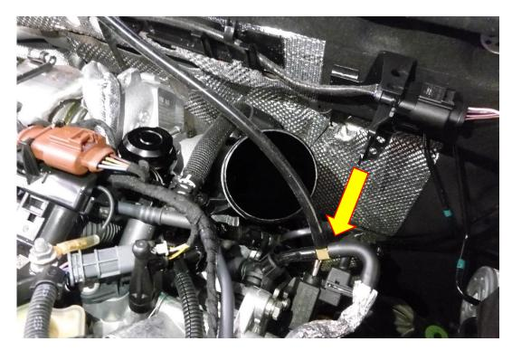
11. The next set of pictures are for illustration purposes - they may not be representative of your engine, but they are the clearest way to show you how to connect your solenoid to the atmospheric or recirculating valve you have fitted. Use the supplied silicone hose to do this, use a sharp knife or side cutters to cut the hose to length.
