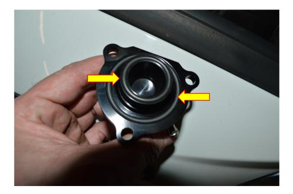
5. Take the Forge Motorsport valve and mount it into position where the OE valve used to be. Use the original T30 Torx fasteners to secure it in place.
