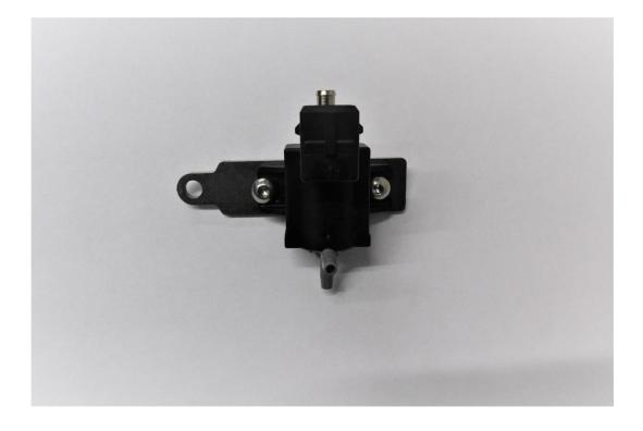
Use a 10mm socket and rachet to attach the supplied M6 fastener, spring washer and solenoid braket to the empty thread at the top of the engine.
