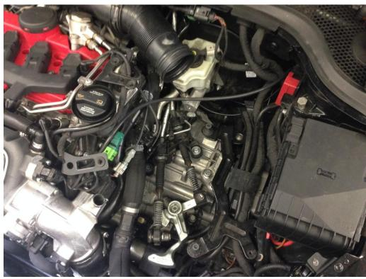
**Step 4** – Locate the shifter cable bracket. Remove mounting bolts
