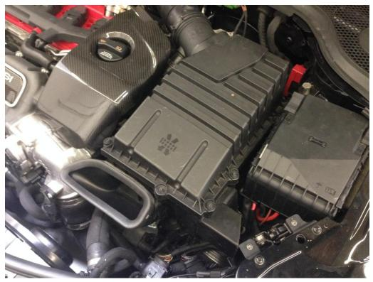
**Step 2** – Remove the carbon piece over the valve cover, around the oil cap. Remove the air duct to the airbox as well. Unclamp the bypass hose and the intake flex hose.
