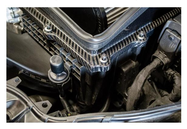
**Step 13 -** Insert intake tube into OE hose at turbo inlet and secure with supplied hose clamp.
