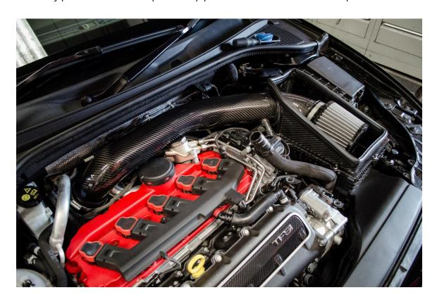
**Step 10** – Install the supplied rubber washers on the factory airbox mounting screws. **Note:** Be sure to install so that the soft, neoprene side faces down.
