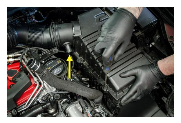
**Step 4** – Using the same set of pliers, loosen the spring clamp at the turbo inlet and slide the clamp up the inlet hose and off the coupler.
