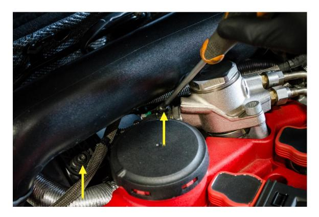
**Step 6** – The inlet pipe should now be loose and able to move freely.
