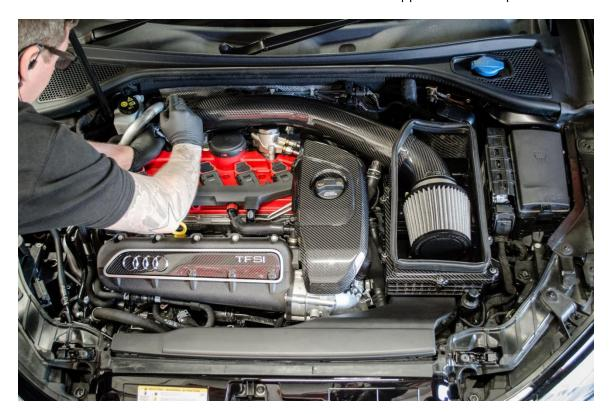
**Step 14 -** Using pliers reinstall the bypass hose and clamp to provision on the 034Motorsport intake tube. Be sure to position OE spring clamp between the 2 white lines on hose.
