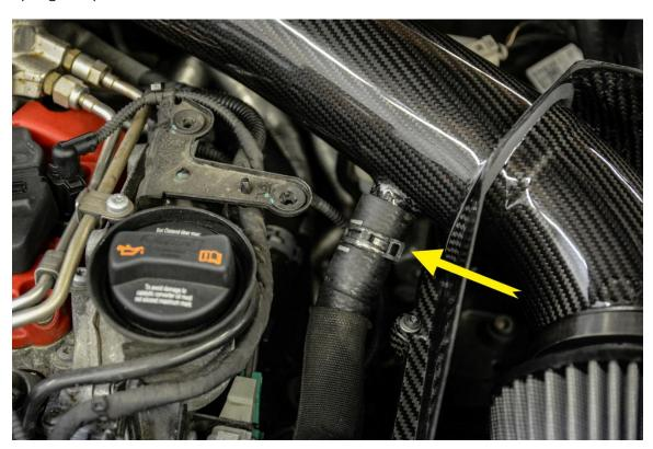
**Step 15** – Using those 2 opposable thumbs again, reinstall the factory carbon fiber trim around the oil fill cap.
