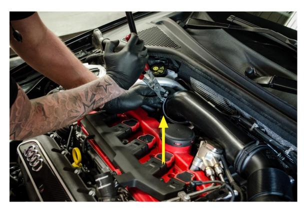
**Step 5** – Using a T30 Torx bit, remove the 2 bolts securing the inlet pipe above the exhaust manifold.
